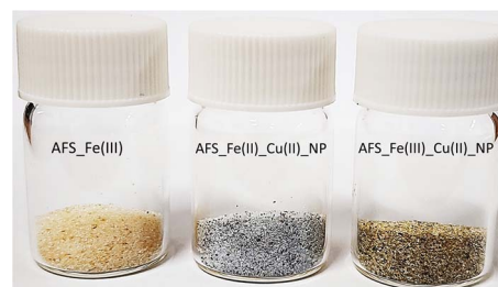
Fig. 2 Optical image showing color variations in amine@silica modified with Fe(III), Fe(II)/Cu(II), and Fe(III)/Cu(II).
