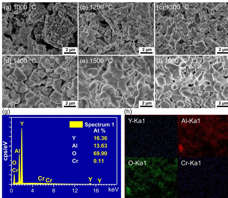
Fig. 3 (a–f) FESEM images of the YAG–YAP:1.3% Cr<sup>3+</sup> sample annealed at different temperatures in the range of 1000–1600 °C (g & h) EDS and EDS mapping spectra of the YAG–YAP:1.3% Cr<sup>3+</sup> sample annealed at 1600 °C.
