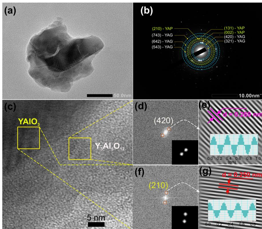
Fig. 4 (a) TEM image, (b) SAED pattern, and (c) high-resolution TEM (HR-TEM) magnified image confirm the coexistence of  $\text{Y}_3\text{Al}_5\text{O}_{12}$  and  $\text{YAlO}_3$  dual-phase structures. (d–g) FFT and IFFT images corresponding to lattice plane fringes of both  $\text{Y}_3\text{Al}_5\text{O}_{12}$  and  $\text{YAlO}_3$  phases.
