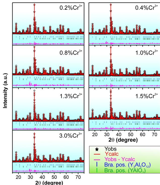
Fig. 2 The Rietveld refinement analysis for YAG–YAP:*x*% Cr<sup>3+</sup> (*x* = 0.2–3.0) samples annealed at 1600 °C for 5 hours in air.
