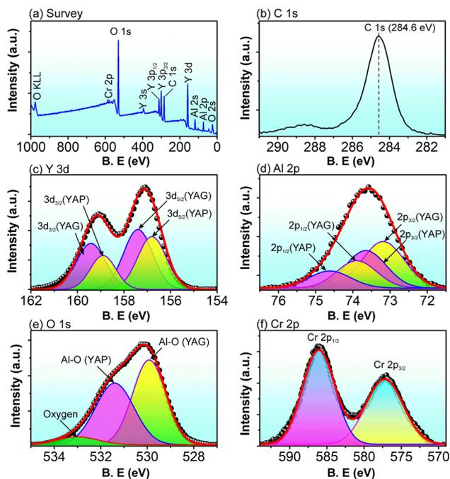
Fig. 5 XPS spectra of  $\text{Y}_3\text{Al}_5\text{O}_{12}$ - $\text{YAlO}_3$ :1.3%  $\text{Cr}^{3+}$  annealed at 1600 °C for 5 h in air: (a) survey, (b) C 1s, (c) Y 3d, (d) Al 2p, (e) O 1s, and (f) Cr 2p.
