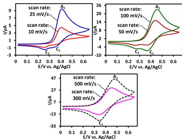
Fig. 1 Cyclic voltammograms of **PTZ** (1.0 mM) in water (acetate buffer,  $c = 0.2$  M, pH = 5.0)/acetonitrile (50 : 50, v/v) at glassy carbon electrode at various scan rates. All voltammograms were recorded at room temperature.
