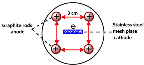
Fig. 6 Cell configuration in electrochemical synthesis of PBP.
