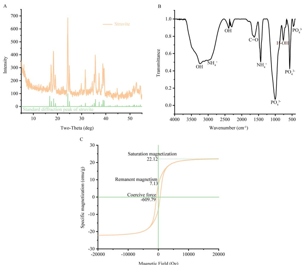
Fig. 2 The physicochemical properties of FSC (A) XRD; (B) FTIR; (C) Hysteresis curve.
