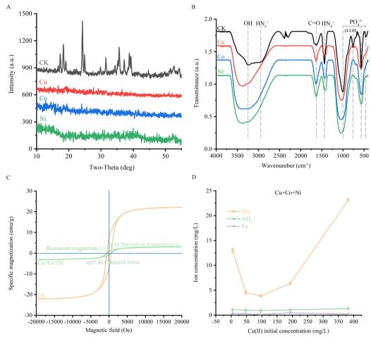
The mechanistic analysis of Cu/Co/Ni passivation by FSC (A) XRD; (B) FTIR; (C) Hysteresis curve; (D) ion release capacity.
