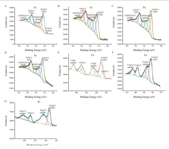
Fig. 7 The XPS of FSC after adsorption of heavy metals (A) Fe2p of FSC; (B) Fe2p of FSC after adsorption of Cu(II); (C) Fe2p of FSC after adsorption of Co(II); (D) Fe2p of FSC after adsorption of Cu(III); (E) Cu2p of FSC after adsorption of Cu(III); (F) Co2p of FSC after adsorption of Cu(III); (G) Ni2p after FSC adsorption of Ni(III).
