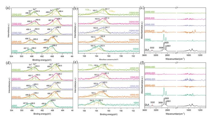
Fig. 3 (a) Sn 3d, (b) S 2p XPS spectra, and (c) FT-IR spectra of OSNS samples. (d) Sn 3d, (e) S 2p XPS spectra, and (f) FT-IR spectra of HSNS samples.
