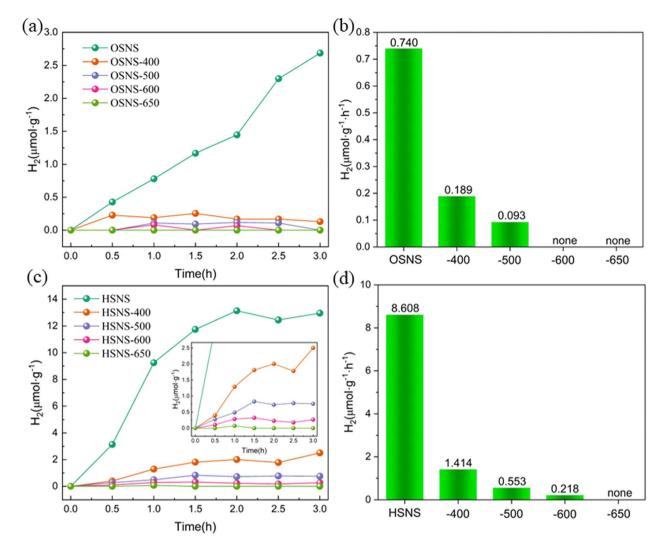
Fig. 6 (a and c) Photocatalytic H<sub>2</sub> production with light radiation time and (b and d) H<sub>2</sub> generation efficiency for OSNS and HSNS before and after annealing.
