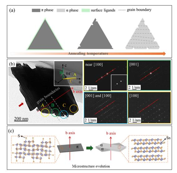
Fig. 5 Schematic illustration of (a) structure evolution of SnS tetrahedrons with increased temperature. (b) TEM image of one SnS tetrahedron (OSNS-650) with various  $\alpha$ -phase grains and their SAED patterns. Inset: Simulated SAED pattern corresponding to area A. (c) Microstructure of  $\pi$  phase and  $\alpha$  phase.
