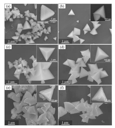
Fig. 1 SEM images of OLA/HMDS-capped SnS particles before and after annealing. (a) OSNS, (b) HSNS, (c) OSNS-400, (d) HSNS-400, (e) OSNS-650 and (f) HSNS-650.
