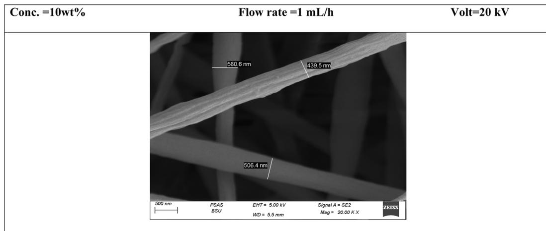
Fig. 10 SEM images for high voltage (20 kV).
