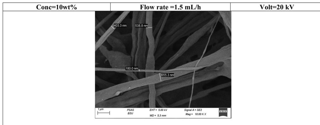
Fig. 7 SEM images for flow rate (1.5 mL h<sup>-1</sup>).
