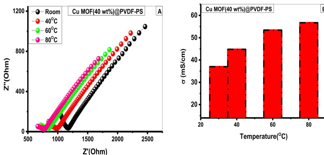
Fig. 33 (A) Nyquist plots of Cu-MOF (40 wt%)@PVDF-PS and (B) the relation between proton conductivity with temperature.
