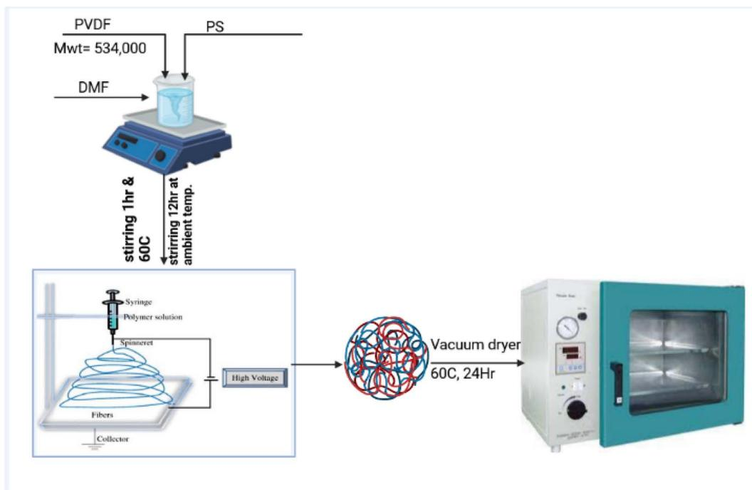
Fig. 1 The preparation method for nano-fiber membranes.
