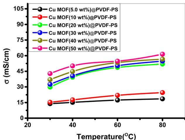
Fig. 35 Variation of proton conductivity ( $\sigma$ ) as a function of temperature for Cu-MOF@PVDF-PS composite membranes with different Cu-MOF loadings (5–50 wt%).
