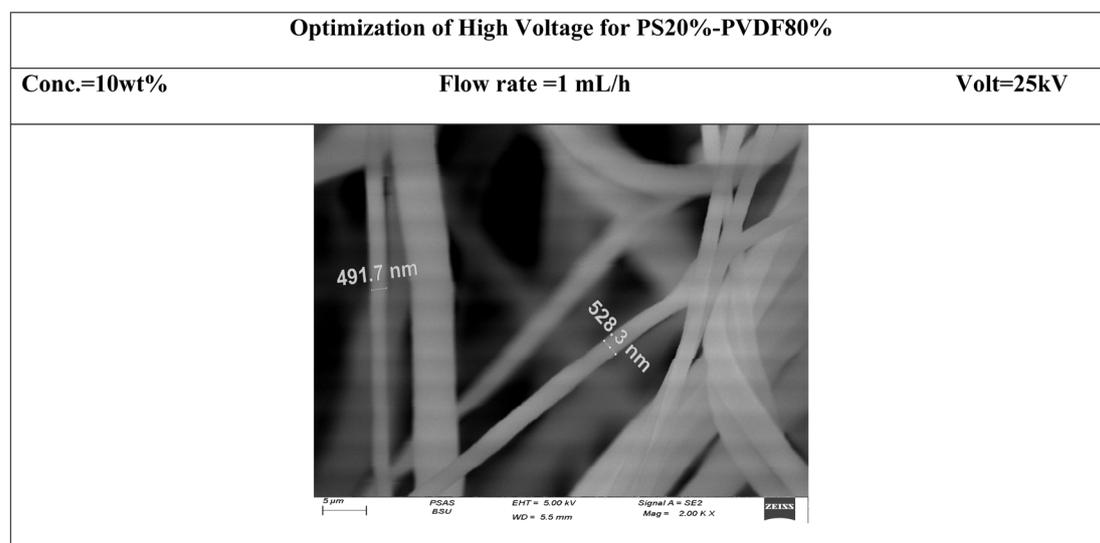
Fig. 9 SEM images for high voltage (25 kV).
