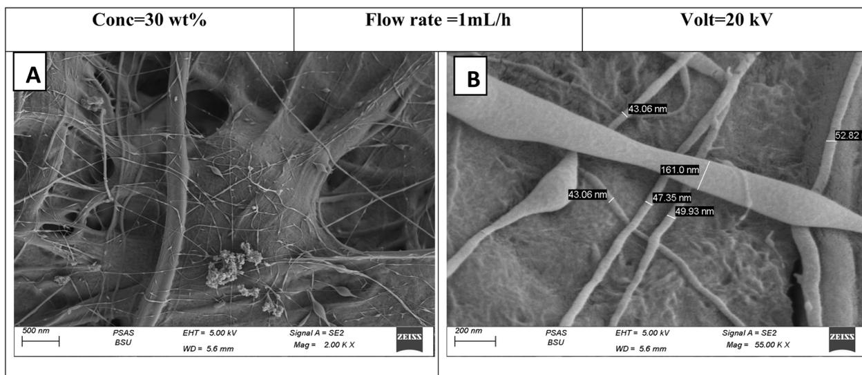
Fig. 6 SEM images of PVDF–PS nanofibers electrospun at 30 wt% total polymer concentration. (A) Morphology revealing dense network with non-uniform diameters and minor bead presence. (B) Detailed view of thickened fibers and partial fusion due to higher solution viscosity.
