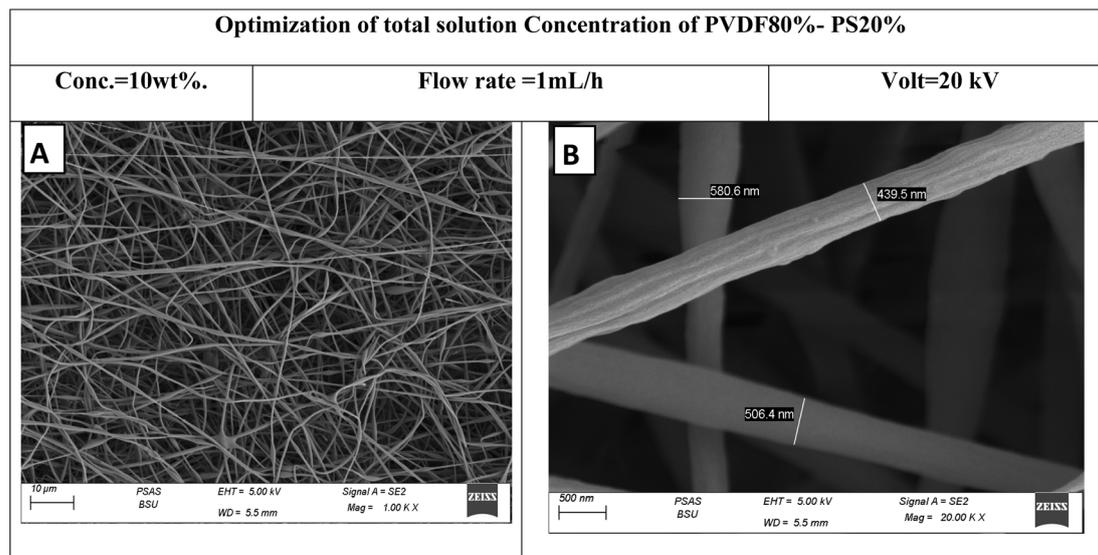
Fig. 3 SEM images of PVDF–PS nanofibers electrospun at 10 wt% total polymer concentration. (A) Low-magnification image showing uniform, continuous fibers without bead formation. (B) Higher magnification revealing smooth surface morphology and consistent diameter distribution.
