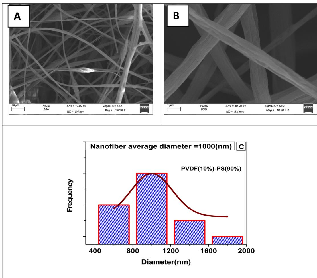
Fig. 11 SEM micrographs of PVDF : PS nanofibers at a 10 : 90 blend ratio. (A) Low-magnification image showing thin, well-aligned fibers with minimal structural defects. (B) High-magnification view highlighting smooth surface morphology and consistent fiber thickness. (C) Histogram showing narrow fiber diameter distribution.
