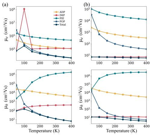
Fig. 6 Electron and hole mobilities ( $\mu_{e_r}$   $\mu_h$ ) vs. temperature for a 2H–InSe monolayer at (a)  $10^{16}$  cm<sup>-3</sup> and (b)  $10^{20}$  cm<sup>-3</sup> carrier concentrations.
