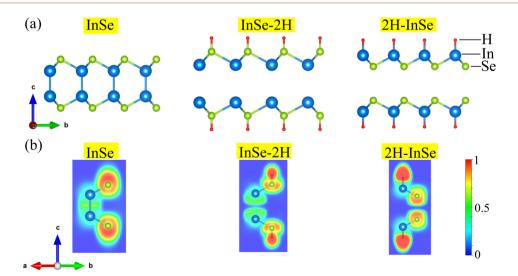
Fig. 1 (a) Side view and (b) electron localization functions (ELF) of a pristine InSe monolayer and its configurations with full hydrogenation on the Se-side (InSe-2H) and the In-side (2H-InSe).
