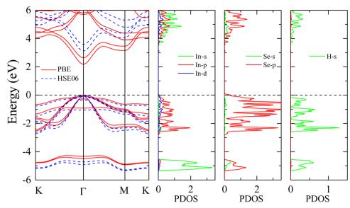
Fig. 3 Band structures of the 2H-InSe monolayer calculated using the PBE method (solid red curves) and the HSE06 hybrid functional (dashed blue curves), along with the partial density of states (PDOS).
