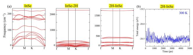
Fig. 2 (a) Phonon dispersion curves of pristine InSe monolayer and fully hydrogenated InSe monolayers with hydrogen atoms adsorbed on the Se sites (InSe–2H) and the In sites (2H–InSe), (b) total energy fluctuation of the 2H–InSe monolayer during AIMD simulation at 300 K.
