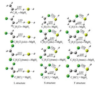
Fig. 3 The directions and the amount of the charge transfer along the  $C(sp^2)-H\cdots H-Mg$  dihydrogen bond and  $H-Mg\cdots Cl$  interaction.
