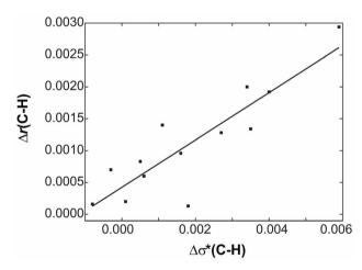
Fig. 2 Correlation between the elongation of the C-H proton-donating bond (in Å) and the increase in electron density within the  $\sigma^*(C-H)$  orbital (in e).
