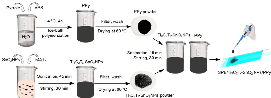
Scheme 1 Graphic representation of the preparation of PPy and \text{Ti}_3\text{C}_2\text{T}_x\text{-SnO}_2 NPs powder for SPE/ \text{Ti}_3\text{C}_2\text{T}_x\text{-SnO}_2 NPs/PPy fabrication.
