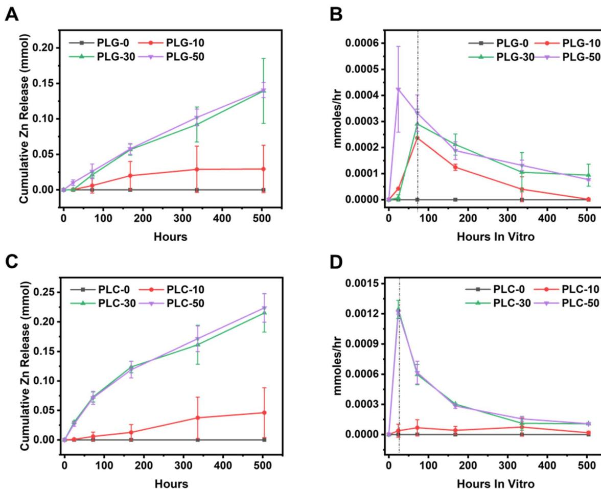
Fig. 6 Study of degradation and release of  $\text{Zn}^{2+}$  *in vitro*. Cumulative  $\text{Zn}^{2+}$  release from PLG-Zn (A) and PLC-Zn (C) nanofiber meshes. Hourly Zn release rates for PLG-Zn (B) and PLC-Zn (D) for a 21 day time period. Data are representative of multiple experiments ( $n = 3$ ).
