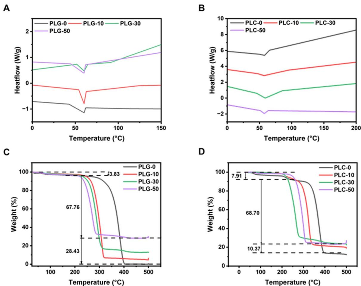
Fig. 4 Thermal analysis of PLG-Zn and PLC-Zn conducted by DSC and TGA respectively. (A and B) DSC curves showing glass transition ( $T_g$ ) of the respective PLG-Zn and PLC-Zn nanofiber meshes. (C and D) Thermal stability of PLG-Zn and PLC-Zn nanofiber meshes at different temperatures analyzed via TGA.
