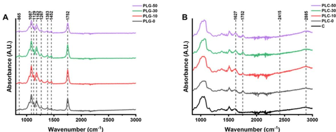
Fig. 3 Chemical composition of the nanofiber meshes. FTIR analysis of chemical compositions of PLG-Zn and PLC-Zn nanofiber meshes (A and B) with different concentrations of Zn NPs. Fig. 4B and C represent the spectra of chitosan.
