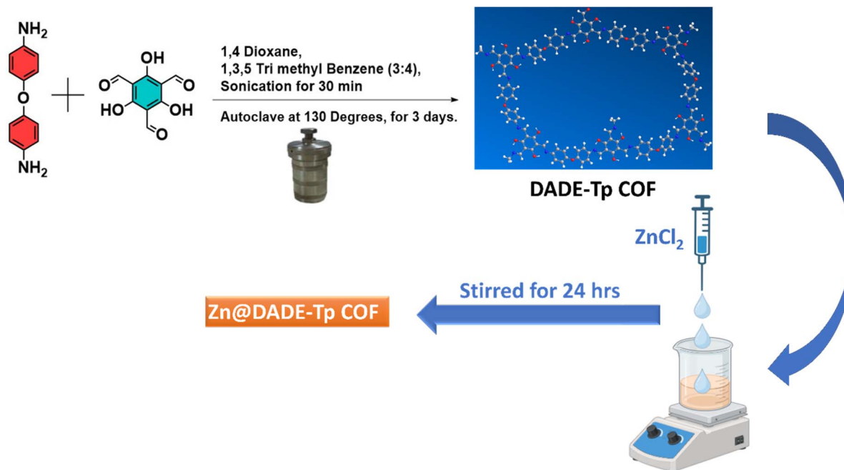
Fig. 1 Synthetic scheme of DADE-Tp COF & Zn@DADE-Tp COF synthesis.
