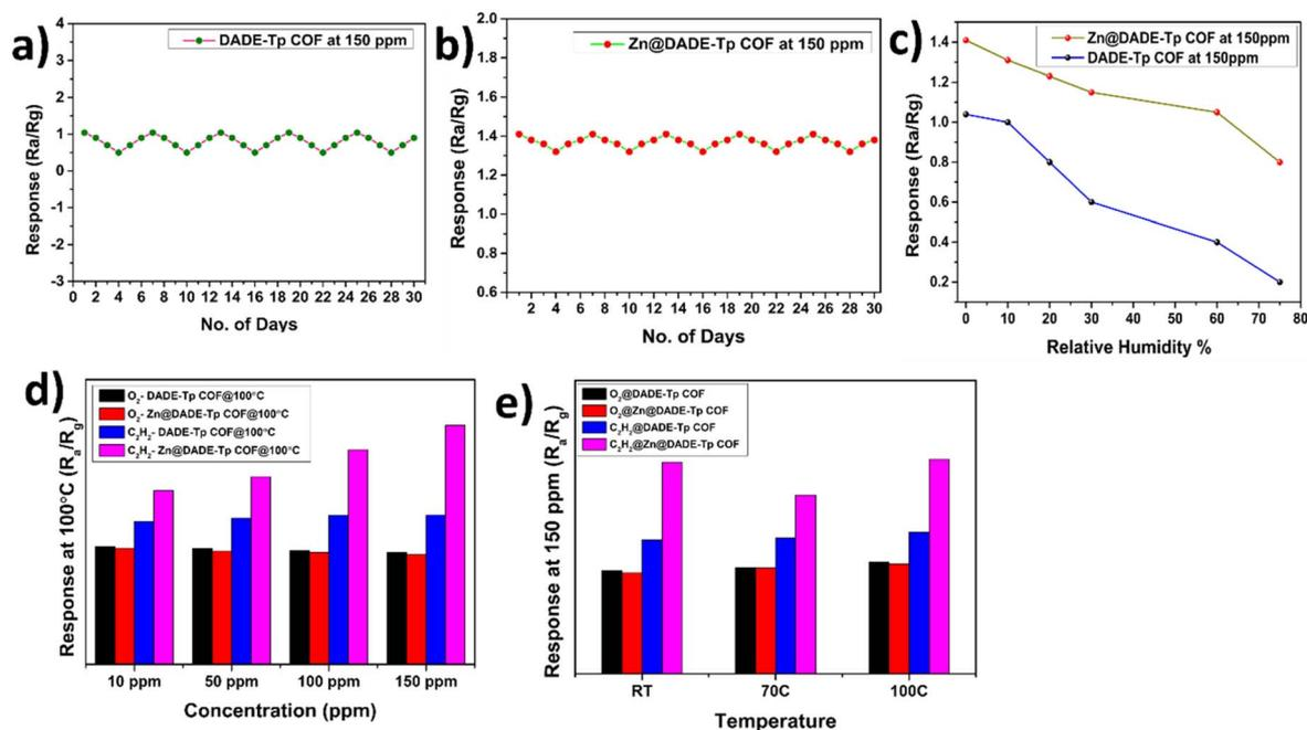
Fig. 6 (a) Stability graph of DADE-Tp COF at 150 ppm, (b) stability graph of Zn@DADE-Tp COF at 150 ppm, (c) relative humidity of DADE-Tp COF and Zn@DADE-Tp COF at 150 ppm, (d) response of DADE-Tp COF and Zn@DADE-Tp COF at 100 °C for all concentrations for oxygen and acetylene sensing (e) response for DADE-Tp COF and Zn@DADE-Tp COF materials at 150 ppm for all the testing temperatures for oxygen and acetylene sensing.
