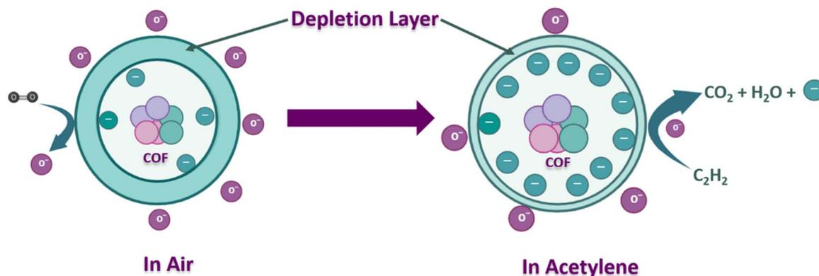
Fig. 7 Schematic illustration of the gas sensing mechanism.
