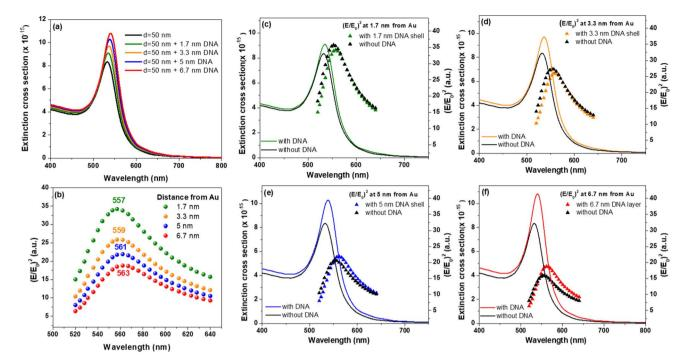
(a) FDTD simulated extinction cross-sections of 50 nm diameter AuNS coated with DNA of different thickness. (b) Value of  $(E/E_0)^2$  at the DNA shell-water interface at different wavelengths in the 520-640 nm interval. (c)-(f) Superposition of extinction band corresponding to 50 nm AuNS without/with DNA shell and  $(E/E_0)^2$  at 1.7, 3.3, 5 and 6.7 nm from Au surface in the absence and presence of DNA shell, in the 520–640 nm interval.
