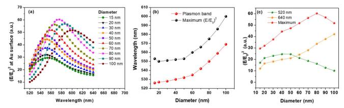
Fig. 2 (a) Value of  $(E/E_0)^2$  near plain AuNS of different diameters at different wavelengths in the 520–640 nm interval, (b) position of plasmon band and maximum  $(E/E_0)^2$  as function of AuNS' diameter, (c) value of  $(E/E_0)^2$  near AuNS at 520 nm, 640 nm and at the position of maximum enhancement, as function of diameter.
