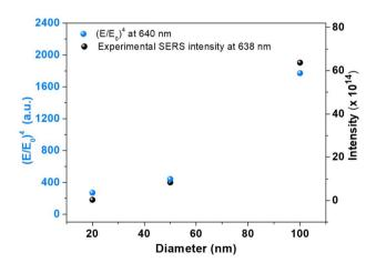
Fig. 5 Comparison between the experimental integrated SERS intensity of the 1075 cm $^{-1}$  band of the 4-MBA obtained for AuNSs of different sizes, under 638 nm, and the FDTD simulated  $(E/E_0)^4$  at 640 nm
