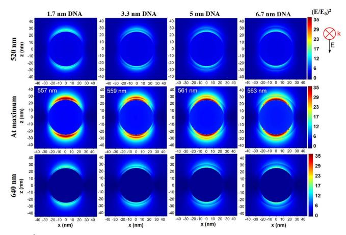
Fig. 7  $(E/E_0)^2$  distribution near the surface of a 50 nm diameter AuNS coated with DNA of different thickness at 520 nm, 640 nm and at the position of maximum field enhancement, at the wavelengths indicated in each image, according to values from Tabel 2.
