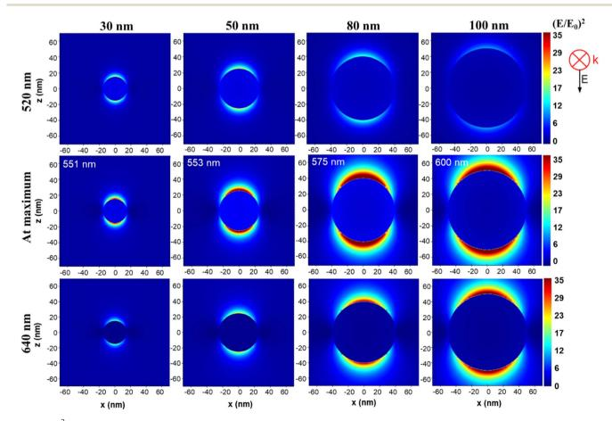
Fig. 3  $(E/E_0)^2$  distribution near the surface of a AuNS with diameter of 30, 50, 80 and 100 nm at 520 nm, 640 nm and at the position of maximum field enhancement, at the wavelengths indicated in each image, according to values from Tabel 1.
