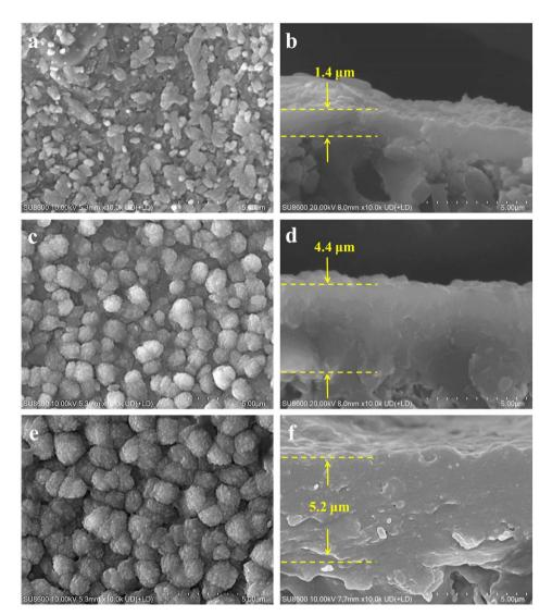
Fig. 6 Surface and cross-sectional SEM images of membranes (MT08, MT09, and MT10) prepared at crystallization times of (a and b) 12 h, (c and d) 36 h, and (e and f) 48 h.
