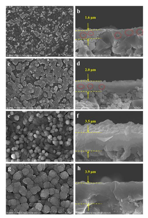
Fig. 4 Surface and cross-sectional SEM images of membranes (MT04, MT05, MT06, and MT07) prepared at crystallization temperatures of (a and b) 150 °C, (c and d) 160 °C, (e and f) 170 °C, and (g and h) 180 °C.
