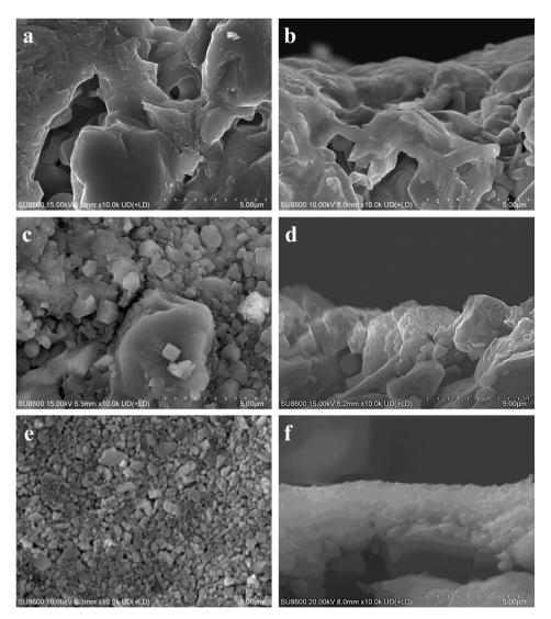
Fig. 1 Surface and cross-sectional SEM images of (a and b) the original macroporous ceramic tube without a seed layer, (c and d) the tube seeded using the hot dip-coating method, and (e and f) the tube seeded using the temperature-varying hot dip-coating method.
