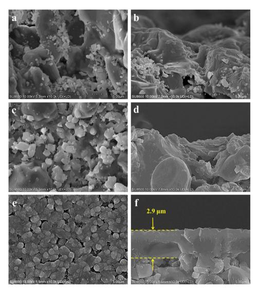
Fig. 2 Surface and cross-sectional SEM images of membranes (MT01, MT02, and MT03) prepared on (a and b) the original macroporous ceramic tube without a seed layer, (c and d) the tube seeded using the hot dip-coating method, and (e and f) the tube seeded using the temp erature-varying hot dip-coating method.
