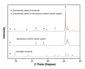
Fig. 3 XRD patterns of (a) simulated mordenite crystals, (b) macroporous ceramic tube, and (c) membrane MT03 prepared on the tube seeded using the temperature-varying hot dip-coating method.
