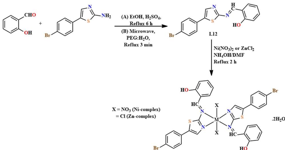
Fig. 15 Synthetic protocol for L12 and [M(L12)<sub>2</sub>(X<sub>2</sub>)]·2H<sub>2</sub>O.
