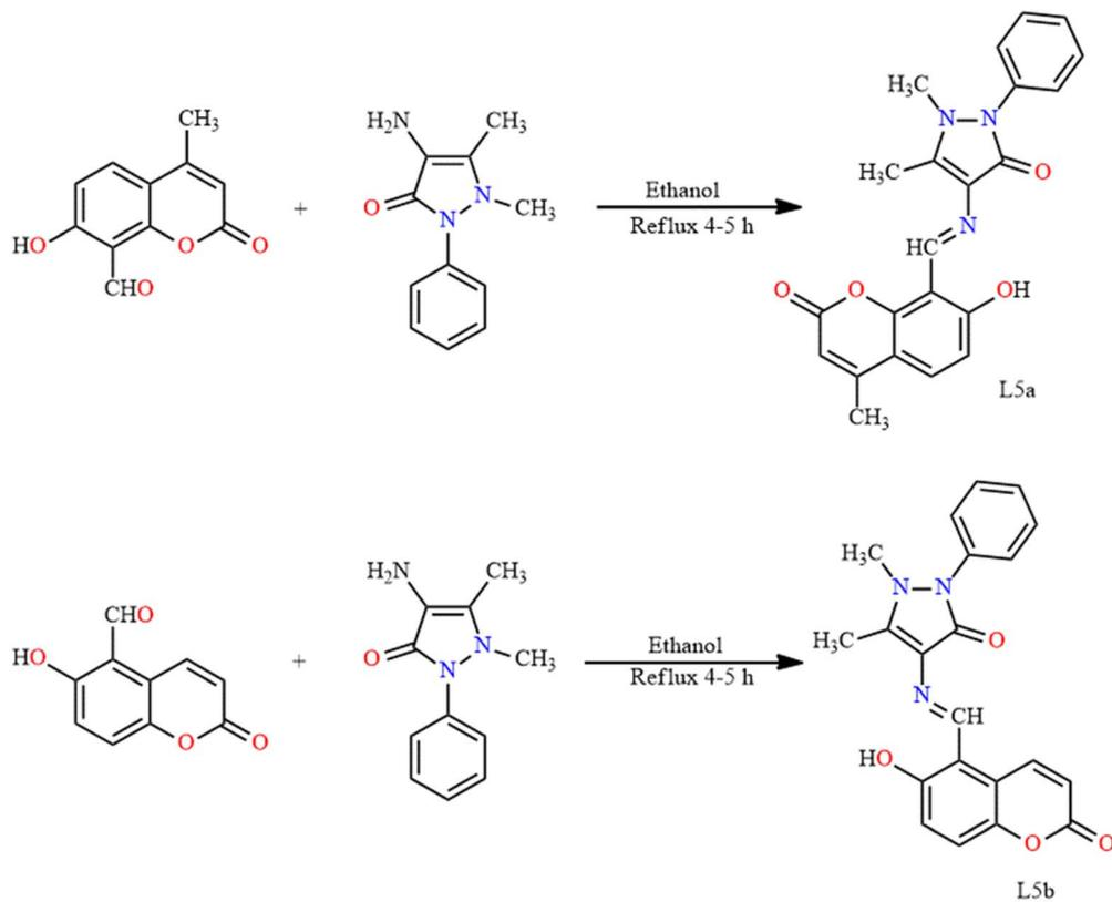
Fig. 6 Synthetic protocol for L5a and L5b.
