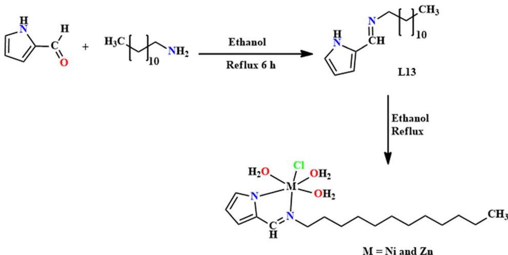
Fig. 16 Synthetic protocol for L13 and [M(L13)Cl·3H<sub>2</sub>O].
