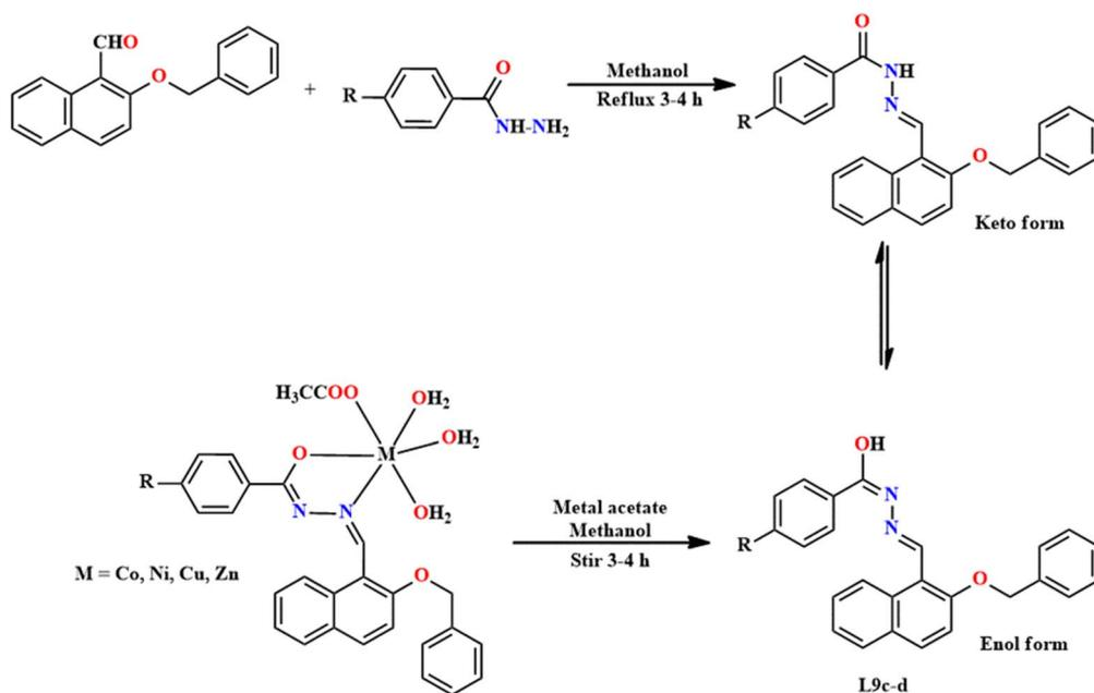
Fig. 12 Synthetic protocol for L9(c–d) and metal complexes.
