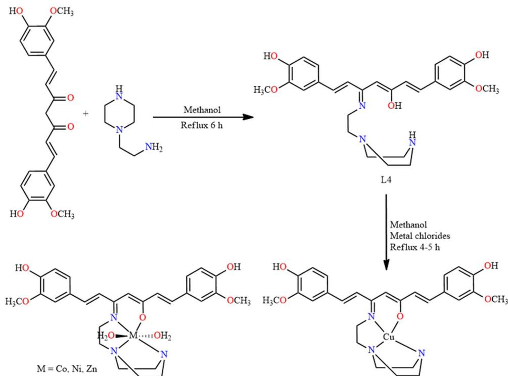
Fig. 5 Synthetic protocol for L4 and metal complexes.
