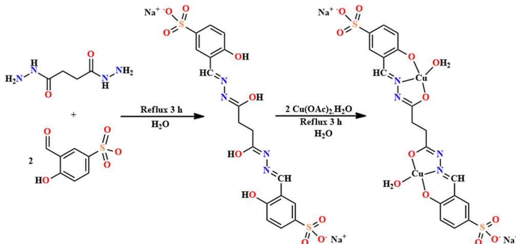
Fig. 19 Synthetic protocol for L15 and (Cu)<sub>2</sub>L15.
