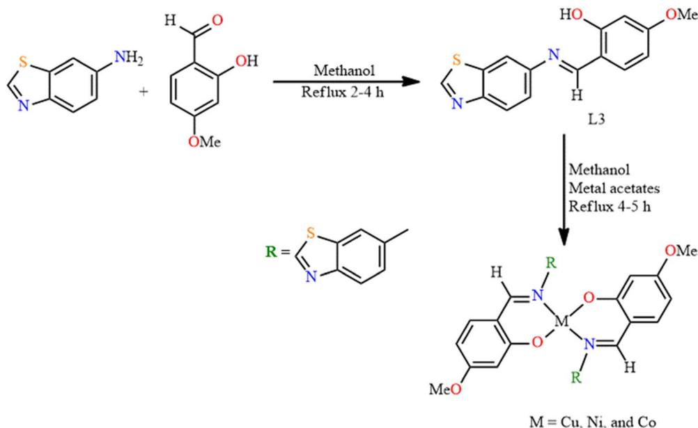
Fig. 4 Synthetic protocol for L3 and metal complexes.
