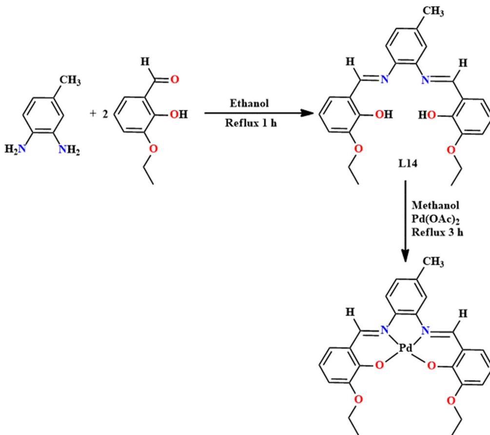
Fig. 18 Synthetic protocol for **L14** and Pd**L14**.
