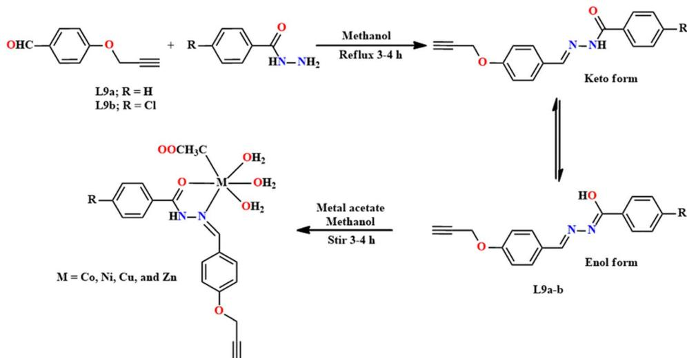
Fig. 11 Synthetic protocol for L9(a–b) and metal complexes.
