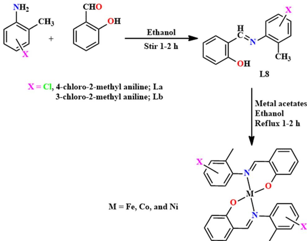
Fig. 10 Synthetic protocol for L8a–b and M(L8a–b)<sub>2</sub>.
