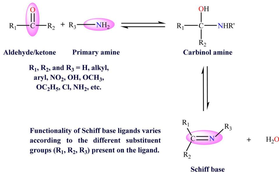
Fig. 1 Schematic representation of Schiff base ligand formation.
