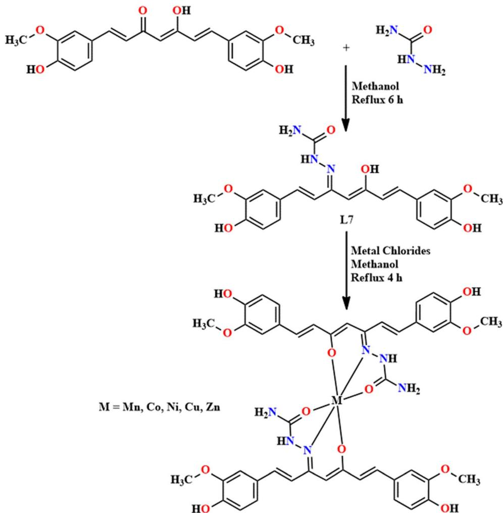
Fig. 9 Synthetic protocol for L7 and M(L7)<sub>2</sub>.
