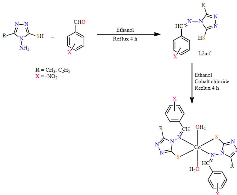
Fig. 3 Synthetic protocol for L2(a–f) and [Co(L2a–f)<sub>2</sub>]<sub>2</sub>H<sub>2</sub>O.
