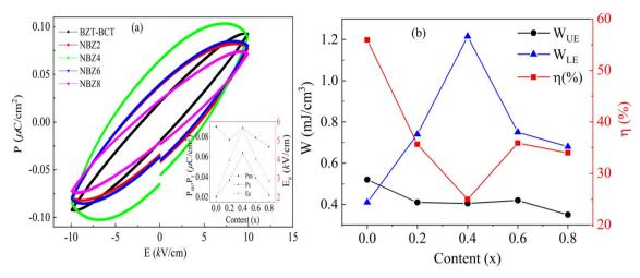
Fig. 5 (a) P(E) curves, (b) the dependences of  $W_{\text{UE}}$ ,  $W_{\text{LE}}$ , and  $\eta_{P-E}$  on NFO content for NFO/BZT-BCT composites. The insert in figure (a) shows the change of  $P_r$ ,  $P_{\text{mr}}$ , and  $E_c$ .
