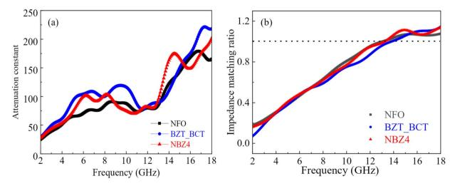
Fig. 10 Frequency dependence of attenuation constant  $\alpha$  (a) and impedance matching ratio (b) of all as prepared samples.
