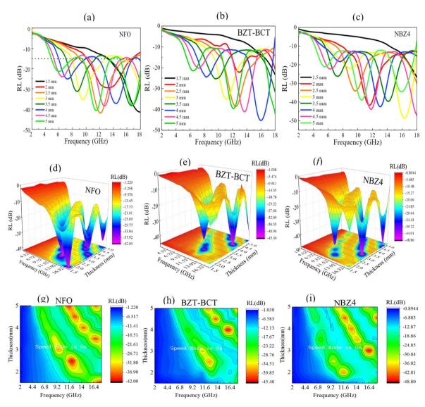
Fig. 9 Two-dimensional RL curves: (a) NFO-parafin; (b) BZT-BCT-parafin; (c) NBZ4-parafin; three-dimensional RL curves: (d) NFO-parafin; (e) BZT-BCT-parafin; (f) NBZ4-parafin; RL contour plots: (g) NFO-parafin; (h) BZT-BCT-parafin; (i) NBZ4-parafin.
