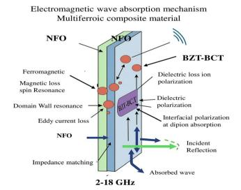
Fig. 11 Diagram illustrating the electromagnetic wave absorption mechanism of NFO/BZT-BCT composites in the  $2-18\ GHz$ .
