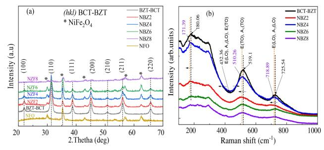
Fig. 1 (a) XRD patterns and (b) Raman spectra of the powdered composites of xNiFe<sub>2</sub>O<sub>4</sub>/(1-x)(0.5Ba( $Zr_{0.2}$ Ti<sub>0.8</sub>)O<sub>3</sub>-0.5(Ba<sub>0.7</sub>Ca<sub>0.3</sub>)TiO<sub>3</sub>).
