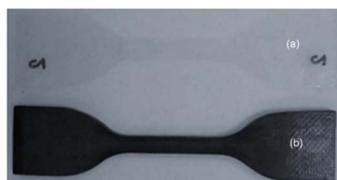
Fig. 3 Tensile test specimens: (a) PE and (b) PVC.
