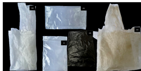
Fig. 2 Plastic samples for characterization: (a) PE, (b) PP, (c) PET, (d) PVC, and (e) PE (LF).
