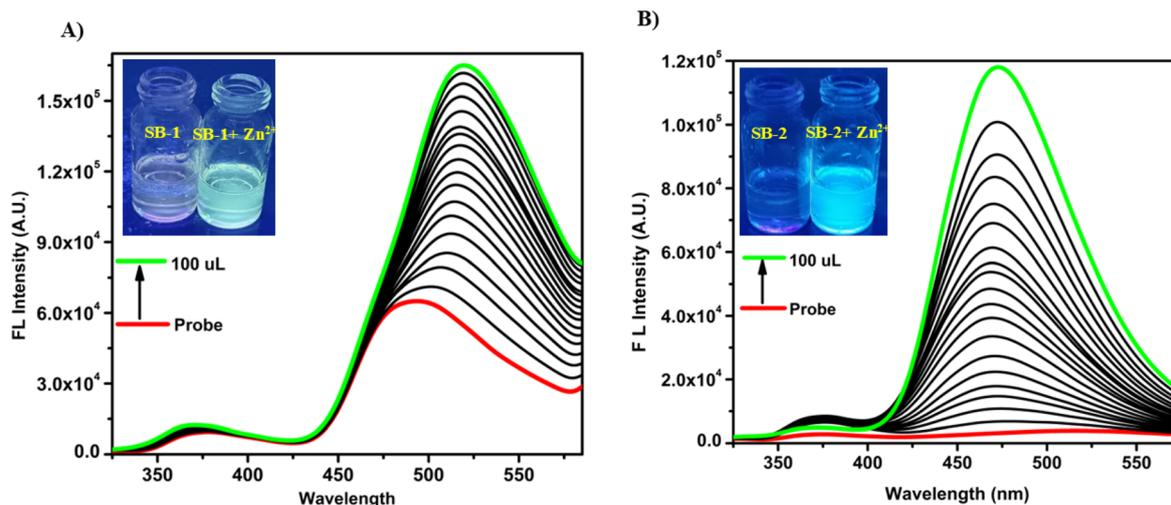
Fig. 3 Emission spectral changes of (A) SB-1 (left,  $10^{-5}$  M) and (B) SB-2 (right,  $10^{-5}$  M) upon the addition of  $\text{Zn}^{2+}$  ions in DMSO. (Inset: photographs captured in DMSO under UV light).
