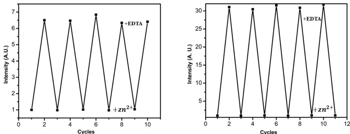
Fig. 8 Reversibility studies of SB-1 (left) and SB-2 (right) were conducted by monitoring fluorescence intensity at 520 nm over five regeneration cycles, with alternating additions of Zn<sup>2+</sup> followed by EDTA.
