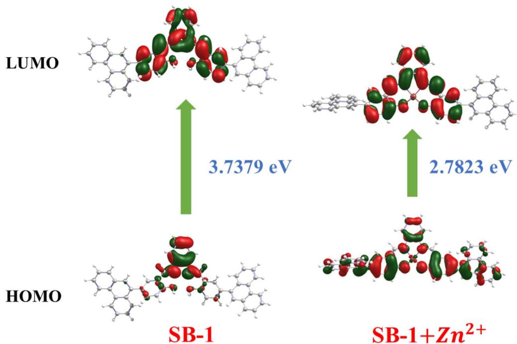
Fig. 7 Selected MOs of SB-1 and SB-1 + Zn<sup>2+</sup> (not to scale; isocontour value = 0.02).
