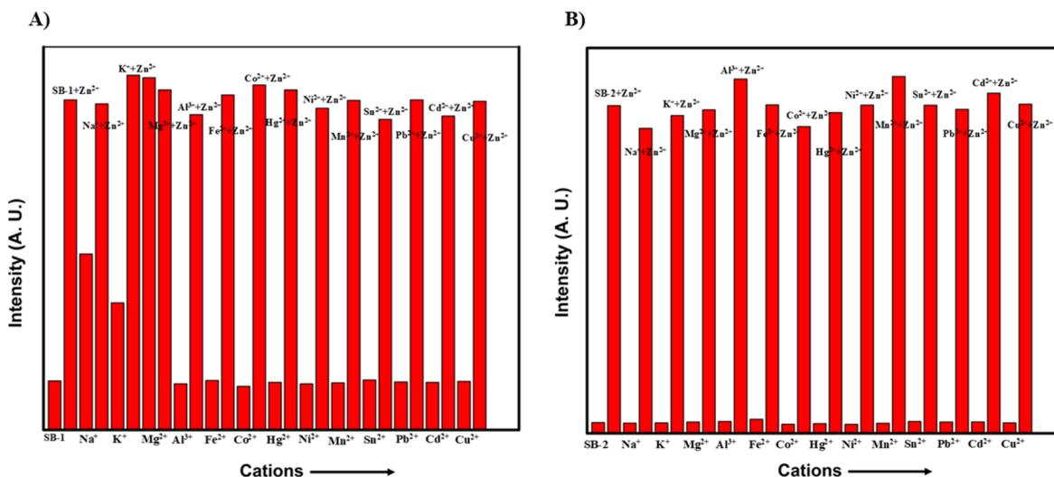
Fig. 5 Examination of competitive studies of SB-1 (A) and SB-2 (B) ( $1 \times 10^{-5}$  M) towards various metal ions. The competitive binding ability of CS-1 and CS-2 ( $1 \times 10^{-5}$  M) in the presence of other interfering metal ions and emission band was monitored at 520 nm.
