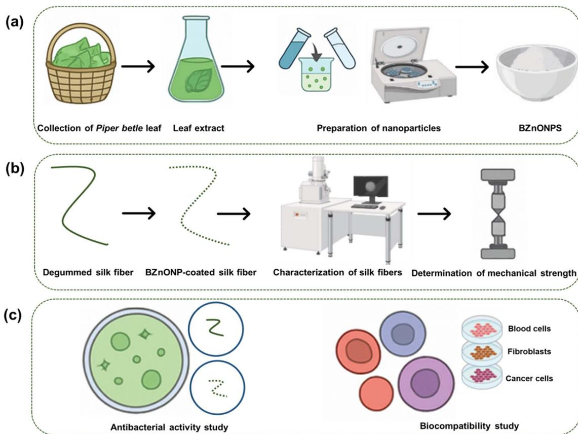
Fig. 1 Schematic illustration of the (a) synthesis of ZnO NPs using *Piper betle* leaf extract. (b) Process involved in the fabrication, characterisation of BZnONP-coated silk fibres and testing of mechanical strength. (c) Functional evaluation of the coated silk fibres for biomedical applications. Prepared using BioRender software.
