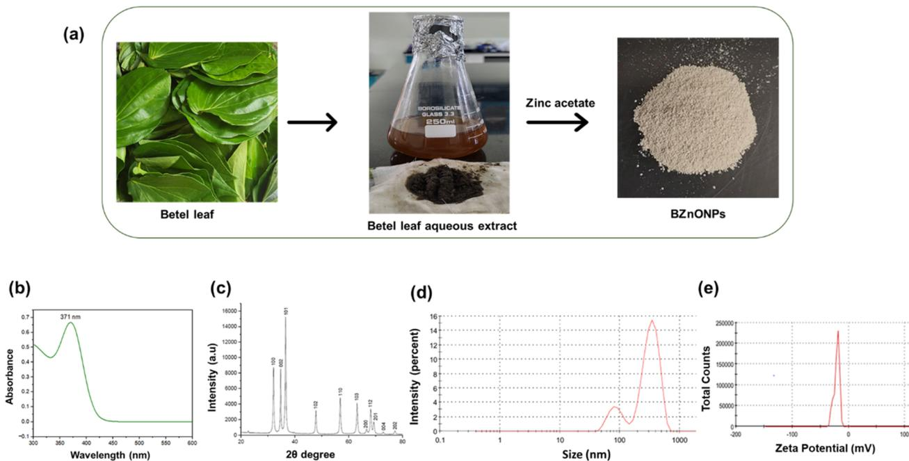
Fig. 2 Biogenic fabrication and characterization of zinc oxide nanoparticles. (a) Schematic representation of the synthesis of zinc oxide nanoparticles using betel leaf extract as a reducing and stabilizing agent (BZnONPs). (b) UV-Visible absorption spectrum of BZnONPs showing a characteristic surface plasmon resonance peak, confirming nanoparticle formation. (c) X-ray diffraction pattern indicating crystalline nature and phase purity. (d) Zeta potential and (e) size analysis of BZnONPs.
