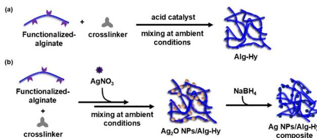
Fig. 1 Schematic illustration of the preparation of Ag NPs-integrated alginate hydrogel material: (a) *in situ* formation of the alginate hydrogel matrix (Alg-Hy) *via* acid-catalysed crosslinking, (b) incorporation of Ag<sub>2</sub>O NPs into the Alg-Hy matrix by mixing precursor solutions under ambient conditions, followed by *in situ* reduction of Ag<sub>2</sub>O NPs to Ag NPs using NaBH<sub>4</sub>.
