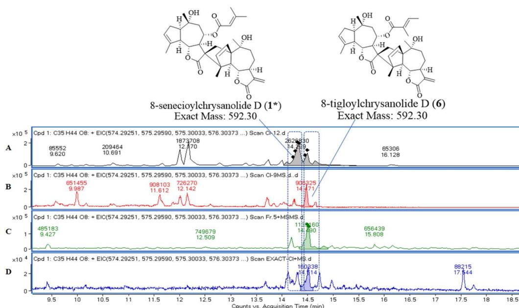
Fig. 8 EIC about molecular formula of C<sub>35</sub>H<sub>44</sub>O<sub>8</sub> (exact mass of *m/z* 590.30). Samples: compound 1 (A); compound 6 (B); fraction 5 (C); *C. indicum* crude extract (D).
