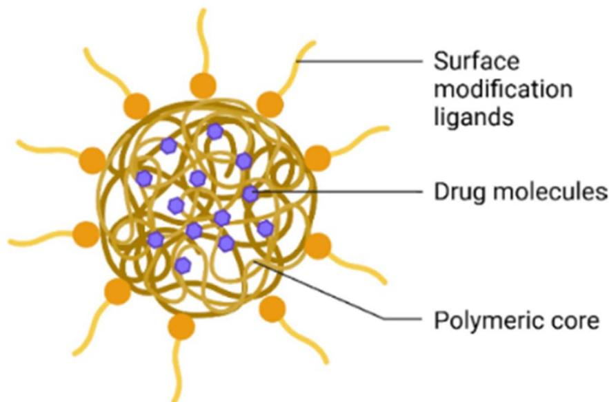
Fig. 2 Basic structure of a polymeric nanoparticle.<sup>35</sup>
