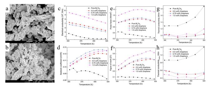
Fig. 6 SEM image of (a) 0.75 (b) 1.5, vol% graphene/Bi<sub>2</sub>Te<sub>3</sub> composite powders; (c–h) represents the thermoelectric properties of samples doped with graphene at different volume fractions and temperatures, (c) conductivity, (d) Seebeck coefficient, (e) power factor, (f) ZT value, (g) thermal conductivity, (h) lattice thermal conductivity. Reproduced from ref. 59 with permission. Copyright 2019 the Elsevier.
