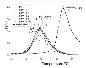
Fig. 7 Temperature dependence of mechanical loss (tan  $\delta$ ) on DMA at a frequency of 10 Hz for PU (1), PHPMA (2), semi-IPNs with the ratio PU/PHPMA = 85/15 (3), and for the nanocomposites containing 1% (4), 3% (5), 5% (6) and 10% (7) of hydroxy-POSS.
