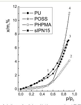
Fig. 1 Isotherms of methylene chloride vapor sorption at 25  $^{\circ}$ C by samples of the native PU (1), native PHPMA (2), semi-IPNs with composition PU/PHPMA = 85/15 (3), by nanofiller hydroxy-POSS (4).
