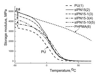
Fig. 11 Temperature dependence of the storage modulus on DMA at a frequency of 10 Hz for PU (1), semi-IPNs with a PU/PHPMA ratio of 85/15 (2) and for the nanocomposites containing 1% (3), 3% (4), 10% (5) of hydroxy-POSS, and of PHPMA (6).
