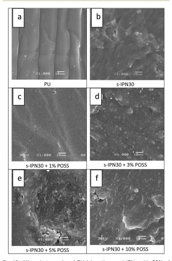
Fig. 15 Microphotographs of PU (a), native semi-IPNs with 30% of PHPMA (b) and nanocomposites based on semi-IPNs with 30% of PHPMA, containing 1% (c), 3% (d), 5% (e) and 10% (f) of POSS at a magnification of 10 000 times.
