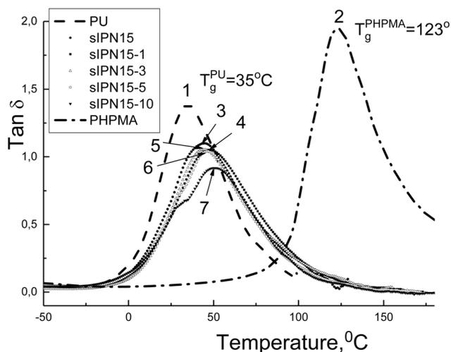
Fig. 7 Temperature dependence of mechanical loss ( $\tan \delta$ ) on DMA at a frequency of 10 Hz for PU (1), PHPMA (2), semi-IPNs with the ratio PU/PHPMA = 85/15 (3), and for the nanocomposites containing 1% (4), 3% (5), 5% (6) and 10% (7) of hydroxy-POSS.
