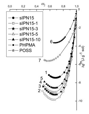
Fig. 3 Concentration dependence of the free energy of polymersolvent mixing for semi-IPNs of the composition PU/PHPMA = 85/15 (1), nanocomposites based on the matrix PU/PHPMA = 85/15, containing 1% (2), 3% (3), 5% (4), 10% (5) of hydroxy-POSS, for PHPMA (6), for nanofiller hydroxy-POSS (7).
