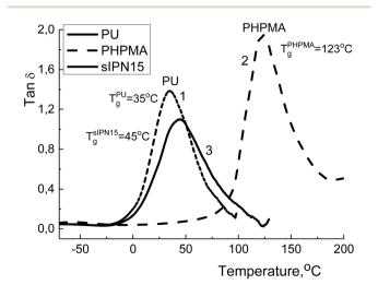
Fig. 6 Temperature dependence of mechanical loss (tan  $\delta$ ) on DMA at a frequency of 10 Hz for the native PU (1), native PHPMA (2) and semi-IPNs with the ratio PU/PHPMA = 85/15 (3).
