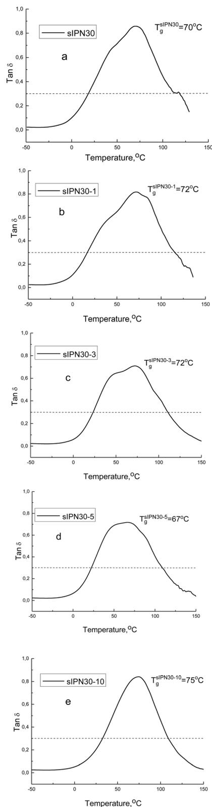
Fig. 9 Temperature dependence of mechanical loss ( $\tan \delta$ ) on DMA at a frequency of 10 Hz for the semi-IPNs samples with a PU/PHPMA ratio = 70/30 (a) and for the nanocomposites containing 1% hydroxy-POSS (b), 3% hydroxy-POSS (c), 5% hydroxy-POSS (d), 10% hydroxy-POSS (e).
