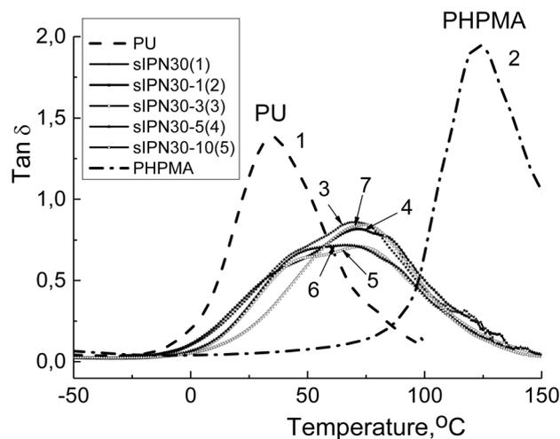
Fig. 8 Temperature dependence of mechanical loss ( $\tan \delta$ ) on DMA at a frequency of 10 Hz for PU (1), PHPMA (2), semi-IPNs with a PU/PHPMA ratio of 70/30 (3), and for the nanocomposites containing 1% (4), 3% (5), 5% (6), 10% (7) of hydroxy-POSS.
