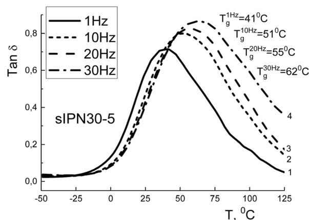
Fig. 10 Temperature dependence of mechanical loss ( $\tan \delta$ ) on DMA at different frequencies for the nanocomposite based on the semi-IPNs matrix with a PU/PHPMA ratio = 70/30, containing 5% hydroxy-POSS: 1 Hz (1), 10 Hz (2), 20 Hz (3), 30 Hz (4).
