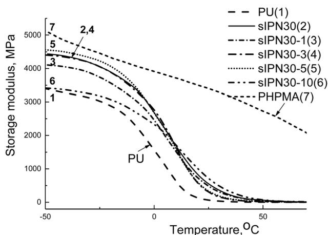
Fig. 12 Temperature dependence of the storage modulus on DMA at a frequency of 10 Hz for PU (1), semi-IPNs with a PU/PHPMA ratio of 70/30 (2) and for the nanocomposites containing 1% (3), 3% (4), 5% (5), 10% (6), and of PHPMA (7).
