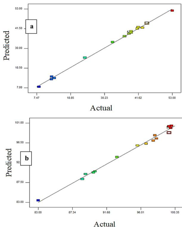
Fig. 3 Actual and forecasted outcomes for the (a) permeate flux % and (b) dye rejection %.
