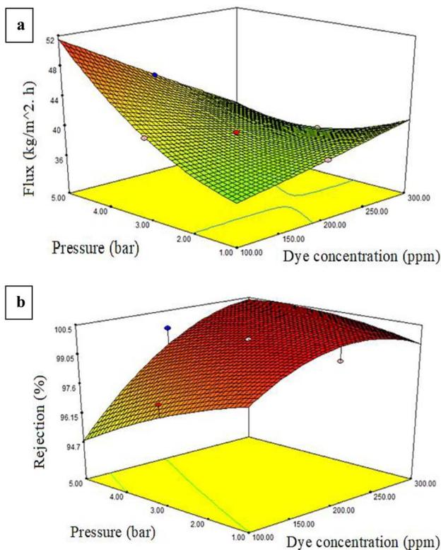
Fig. 8 Effect of dye concentration and pressure on the (a) flux and (b) dye rejection (%) at an additive loading of 44 mg.
