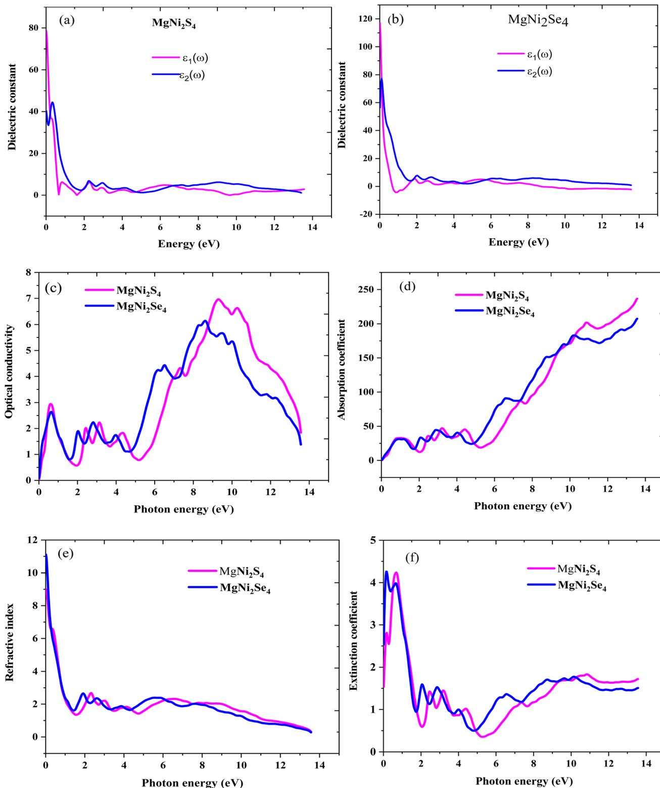
Fig. 6 (a) represents the real part  $\epsilon_1(\omega)$  and imaginary part  $\epsilon_2(\omega)$  of dielectric constant of  $\text{MgNi}_2\text{S}_4$  and (b) represents real part  $\epsilon_1(\omega)$  and imaginary part  $\epsilon_2(\omega)$  of dielectric constant of  $\text{MgNi}_2\text{Se}_4$  (c) represents optical conductivity, (d) represents absorption coefficient (e) represents reflective index and (f) excitation coefficient under GGA-mBJ potential approximation.
