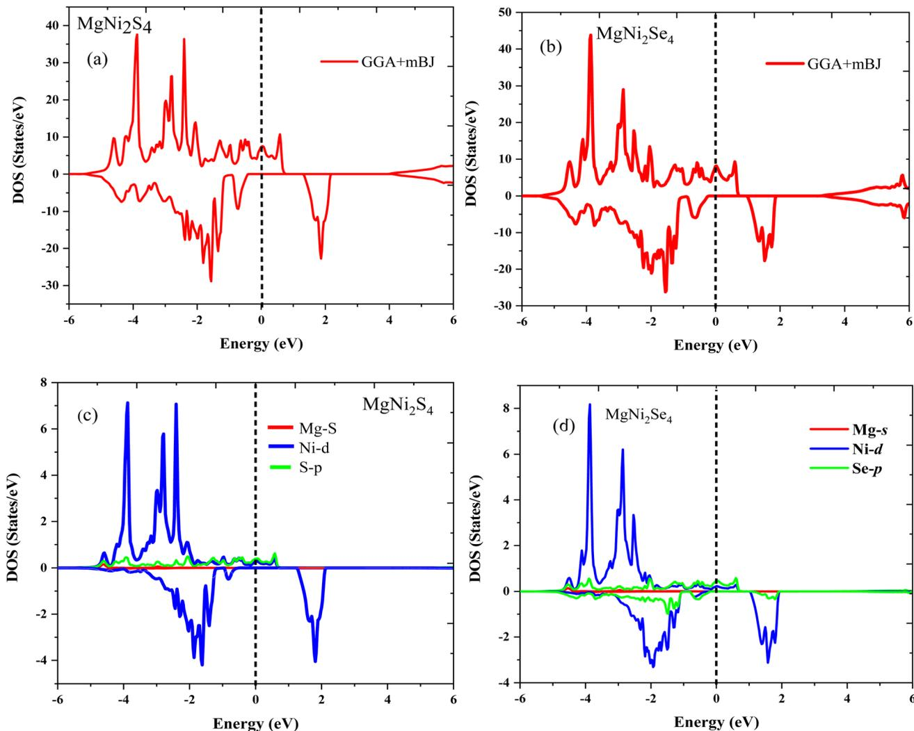
Fig. 5 (a) and (b) represents total density (TDOS) of states in spin up and spin down channels for  $\text{MgNi}_2\text{X}_4$  ( $\text{X} = \text{S}/\text{Se}$ ) and (c) and (d) represents partial density of states in spin up and spin down channels for  $\text{MgNi}_2\text{X}_4$  ( $\text{X} = \text{S}/\text{Se}$ ) respectively under GGA-mBJ potential approximation.
