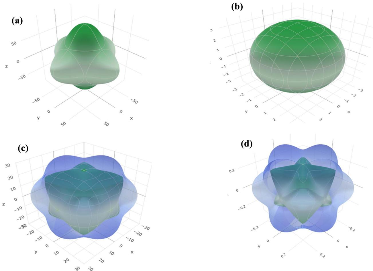
Fig. 10 (a–d) Directional dependence of (a) Young's modulus ( $Y$ ), (b) linear compressibility ( $\beta$ ), (c) shear modulus ( $G$ ), and (d) Poisson's ratio ( $\nu$ ) for  $\text{MgNi}_2\text{Se}_4$  compound.
