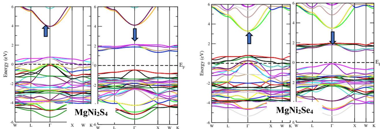
Fig. 4 Plot of the electronic band structure for  $\text{MgNi}_2\text{X}_4$  ( $\text{X} = \text{S}/\text{Se}$ ) in spin up and spin down channels under GGA + mBJ potential approximation.
