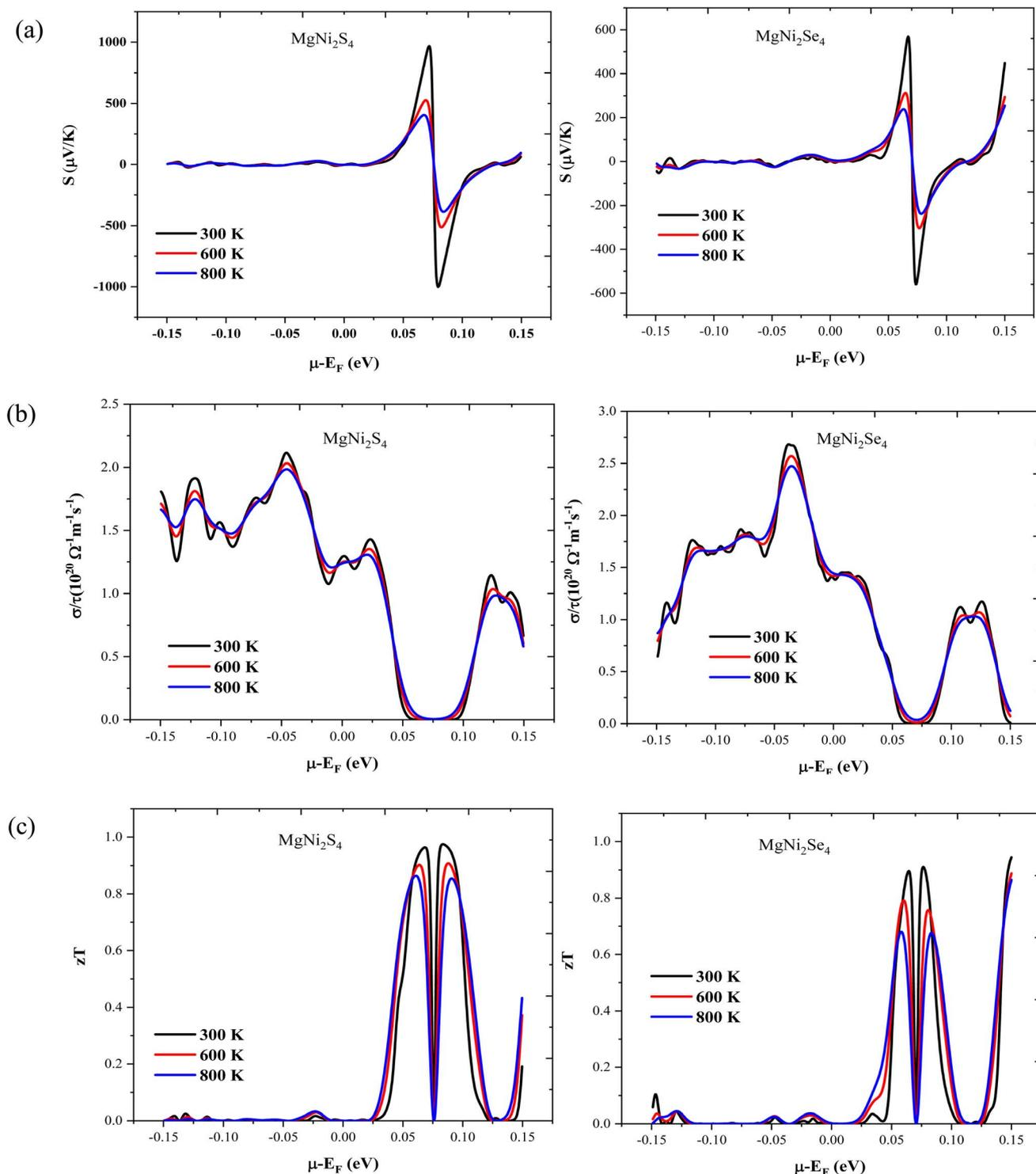
Fig. 8 (a–c) Thermoelectric parameters (a) Seebeck coefficient, (b) electrical conductivity and figure of merit ( $zT$ ) against chemical potential.
