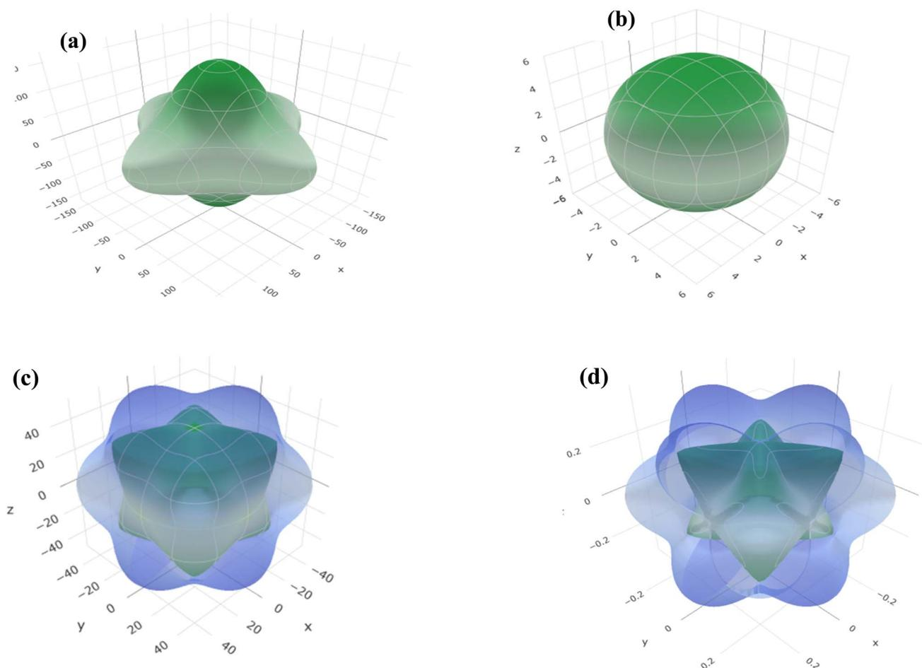
Fig. 9 (a–d) Directional dependence of (a) Young's modulus ( $Y$ ), (b) linear compressibility ( $\beta$ ), (c) shear modulus ( $G$ ), and (d) Poisson's ratio ( $\nu$ ) for MgNi<sub>2</sub>S<sub>4</sub> compound.
