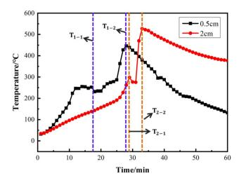
Fig. 8 Partial temperature characteristics of LFP under heat radiation intensities of  $1.88~\rm kW~m^{-2}$  and  $1.57~\rm kW~m^{-2}$ .
