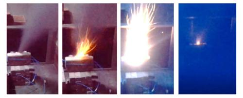
Fig. 5 Thermal runaway phenomenon in NCM.
