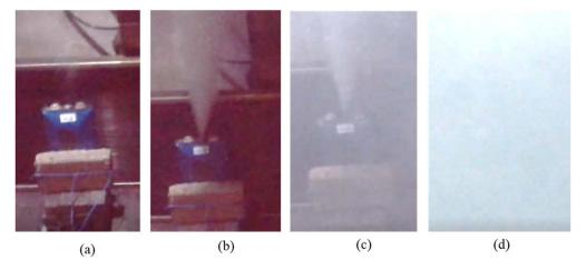
Fig. 9 Thermal runaway phenomenon in LFP (a) LFP without thermal runaway, (b) LFP safety valve opening, (c) rapid smoke ejection, (d) entire space filled with smoke.
