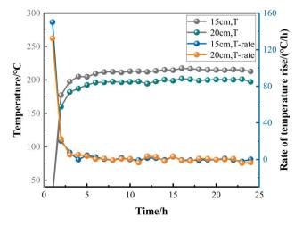
Fig. 7 Temperature characteristics of LFP under heat radiation intensities of  $1.88~\rm kW~m^{-2}$  and  $1.57~\rm kW~m^{-2}$  after enduring for 24 h.
