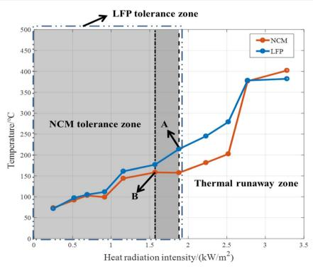
Fig. 11 Heat radiation tolerance zone.
