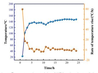
Fig. 4 Temperature characteristics of NCM under a heat radiation intensity of 1.158 kW  $\rm m^{-2}$  after enduring for 24 h.
