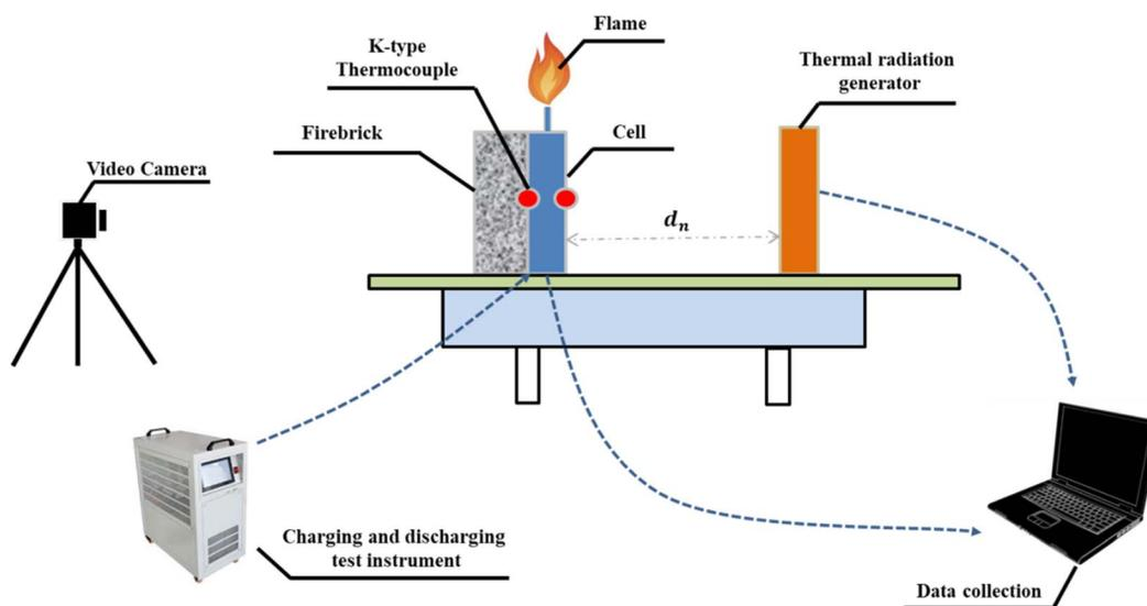
Fig. 2 Thermal radiation field test platform layout.
