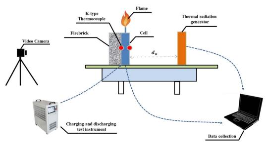
Fig. 2 Thermal radiation field test platform layout.
