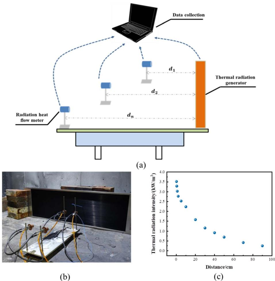
Fig. 1 Thermal radiation field test platform layout (a) schematic, (b) real diagram, (c) correspondence between thermal radiation and distance.
