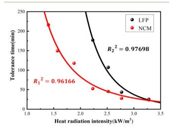
Fig. 10 Thermal radiation-endurance time data fitting curve of the lithium battery.
