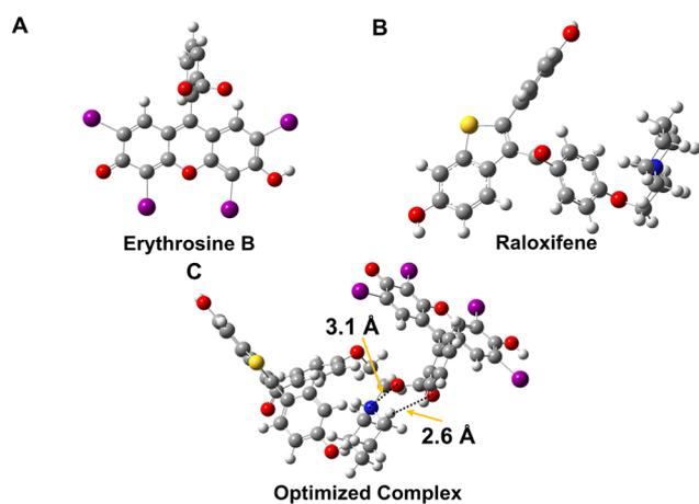
Fig. 3 (A) Optimized structure of erythrosine B shows the xanthene ring system with iodine atoms and carboxylate group; (B) optimized structure of raloxifene highlighting the benzothiophene scaffold, phenolic groups, and piperidine moiety; (C) optimized geometry of the erythrosine B–raloxifene complex shows key binding interactions, including hydrogen bonding (2.6 Å) and electrostatic attraction (3.1 Å).
