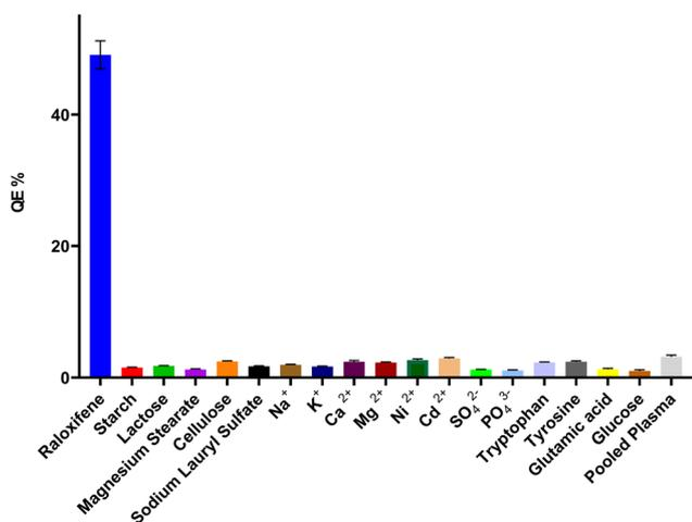
Fig. 5 Selectivity studies show the quenching efficiency percentage (QE%) of various potential interferents compared to raloxifene (1.5  $\mu\text{g mL}^{-1}$ ), demonstrating high selectivity with interferent responses below 3% versus 48% for raloxifene under identical conditions. Error bars represent standard deviation from triplicate measurements ( $n = 3$ ).
