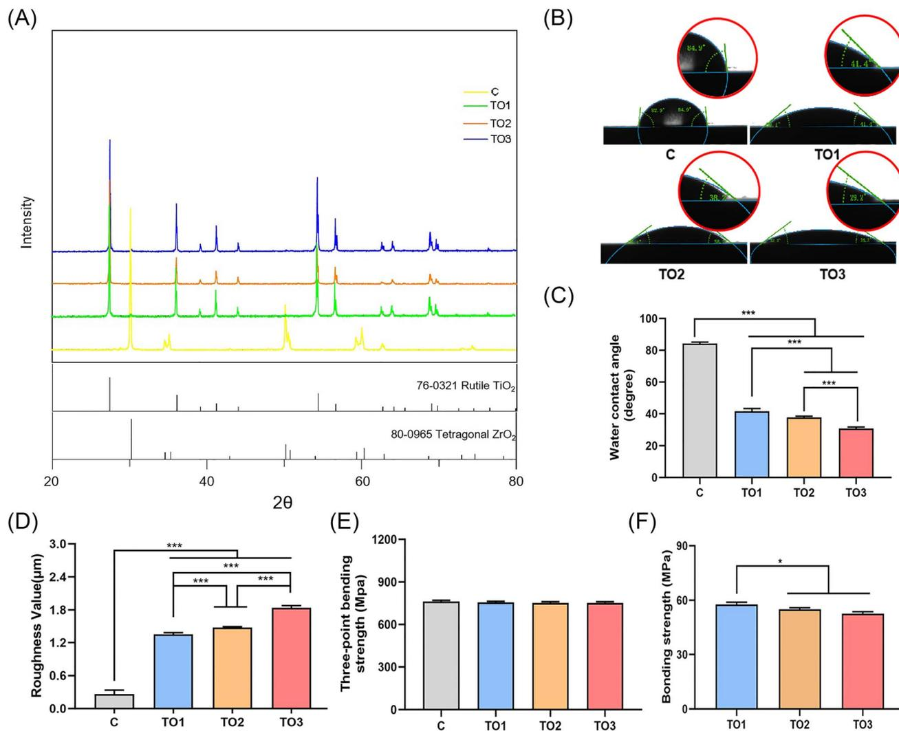
Fig. 3 (A) XRD patterns of different samples. (B and C) Water contact angles of each group zirconia. (D) Surface roughness value of the C, TO<sub>1</sub>, TO<sub>2</sub>, and TO<sub>3</sub> groups. (E) Three-point bending strength of the specimens. (F) Bonding strength of coatings from each group of samples. \* $P < 0.05$ , \*\* $P < 0.01$ , \*\*\* $P < 0.001$ .
