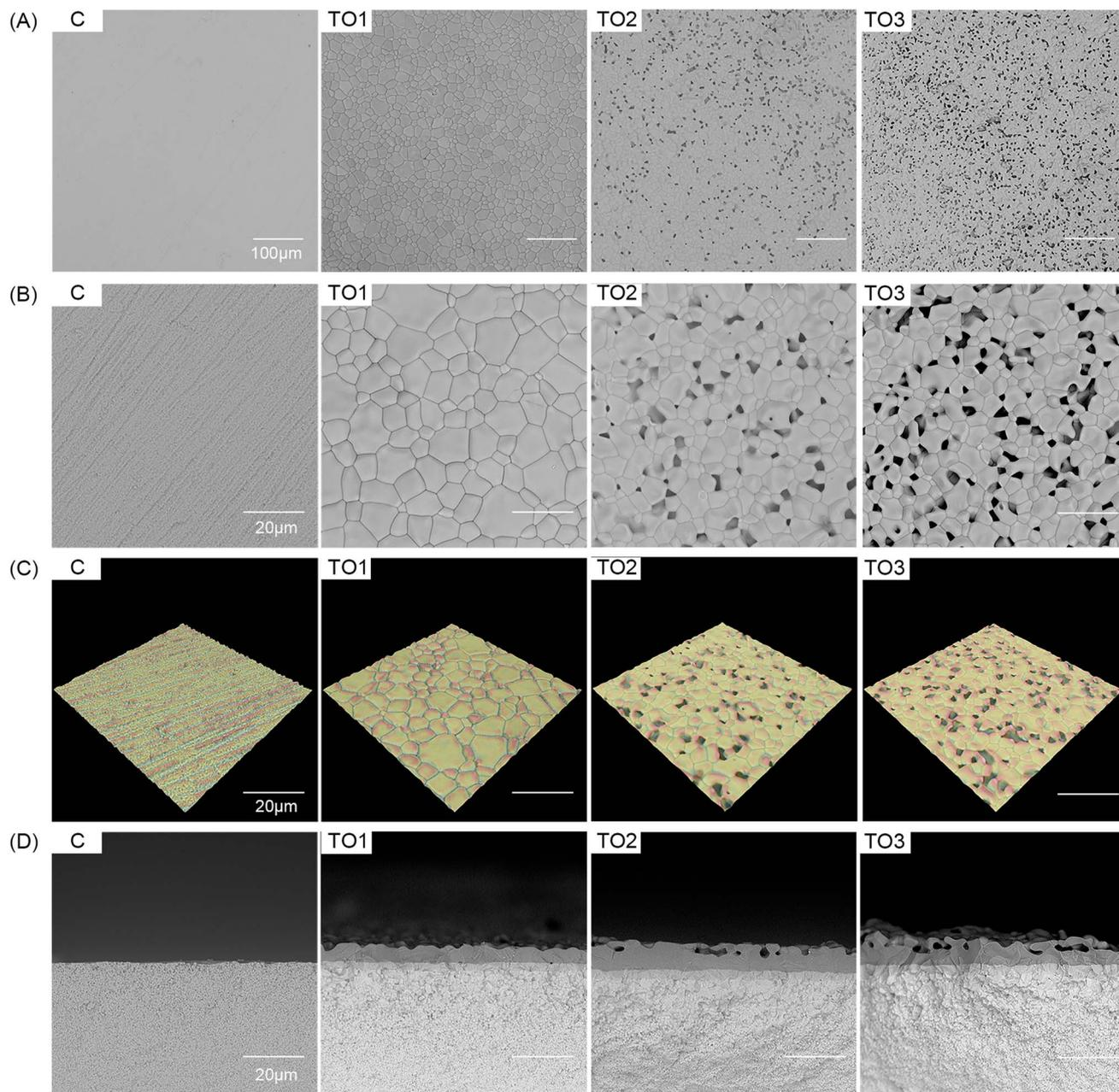
Fig. 1 SEM images of the samples: (A) low magnification (scale bar: 100  $\mu\text{m}$ ), (B) high magnification (scale bar: 20  $\mu\text{m}$ ). (C) 3-D reconstruction images of zirconia specimens in each group. (D) Cross-sectional SEM images of zirconia samples from different groups.
