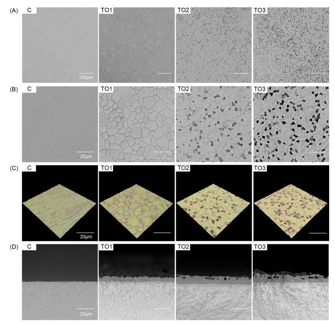
Fig. 1 SEM images of the samples: (A) low magnification (scale bar:  $100 \mu m$ ), (B) high magnification (scale bar:  $20 \mu m$ ). (C) 3-D reconstruction images of zirconia specimens in each group. (D) Cross-sectional SEM images of zirconia samples from different groups.
