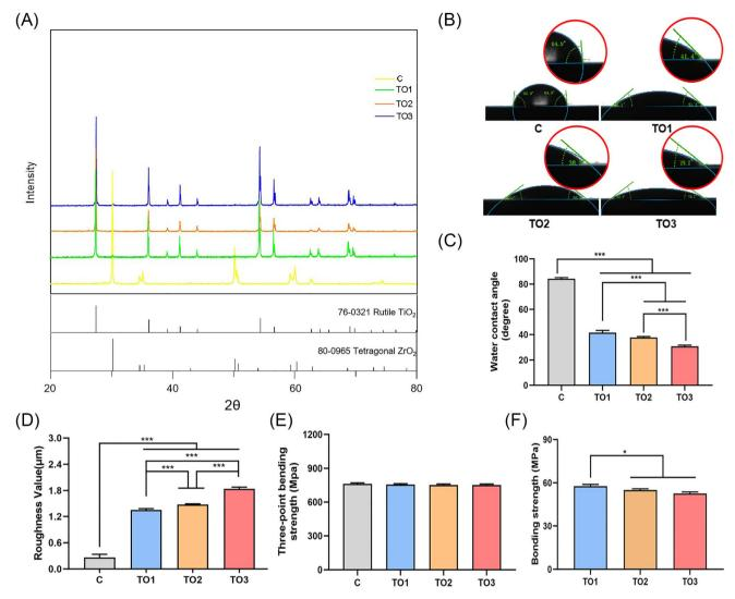
Fig. 3 (A) XRD patterns of diffrernt samples. (B and C) Water contact angles of each group zirconia. (D) Surface roughness value of the C,  $TO_1$ ,  $TO_2$ , and  $TO_3$  groups. (E) Three-point bending strength of the specimens. (F) Bonding strength of coatings from each group of samples. \*P < 0.05, \*\*P < 0.01, \*\*\*P < 0.001.
