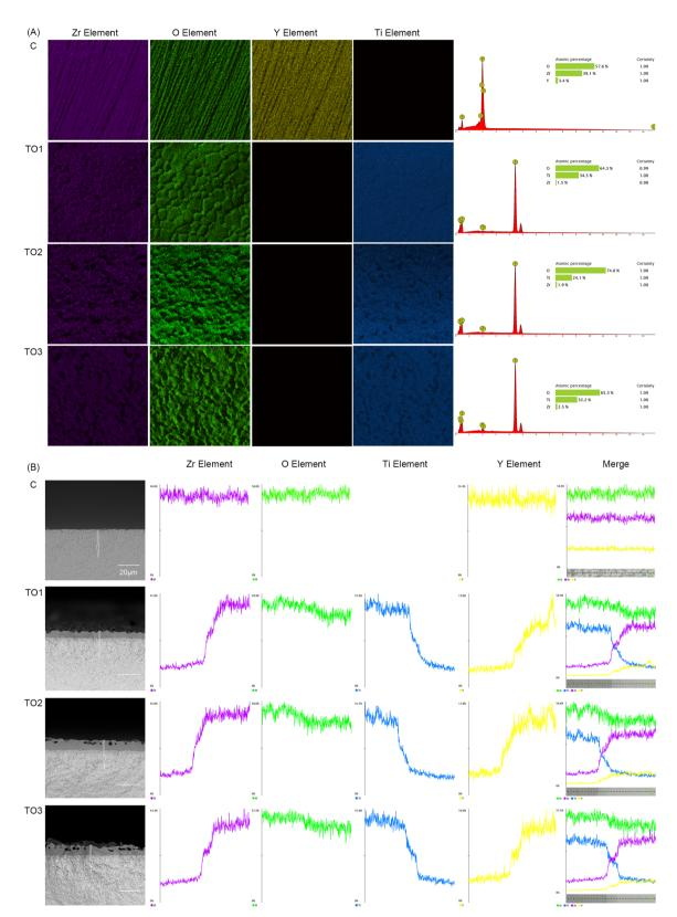
Fig. 2 (A) Elemental mapping of zirconia specimen surfaces in each group. (B) The EDS line-scanning results of longitudinal sections of zirconia.
