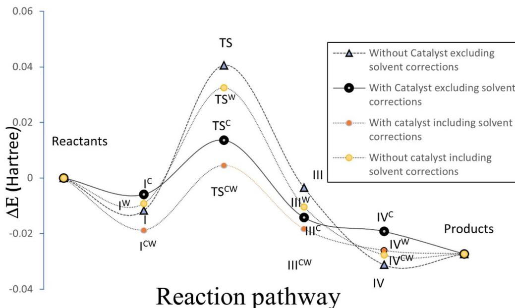
Fig. 4 The energy profile diagram of the reaction showing relative energies (in Hartree) at different stage of reaction with (I<sup>C</sup>) and without catalyst (I) and also including the effect of solvent (indicated by superscript W) during the course of reaction.
