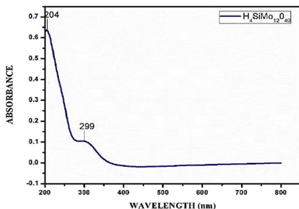
Fig. 2 UV-visible spectrum of aqueous solution of SMA.
