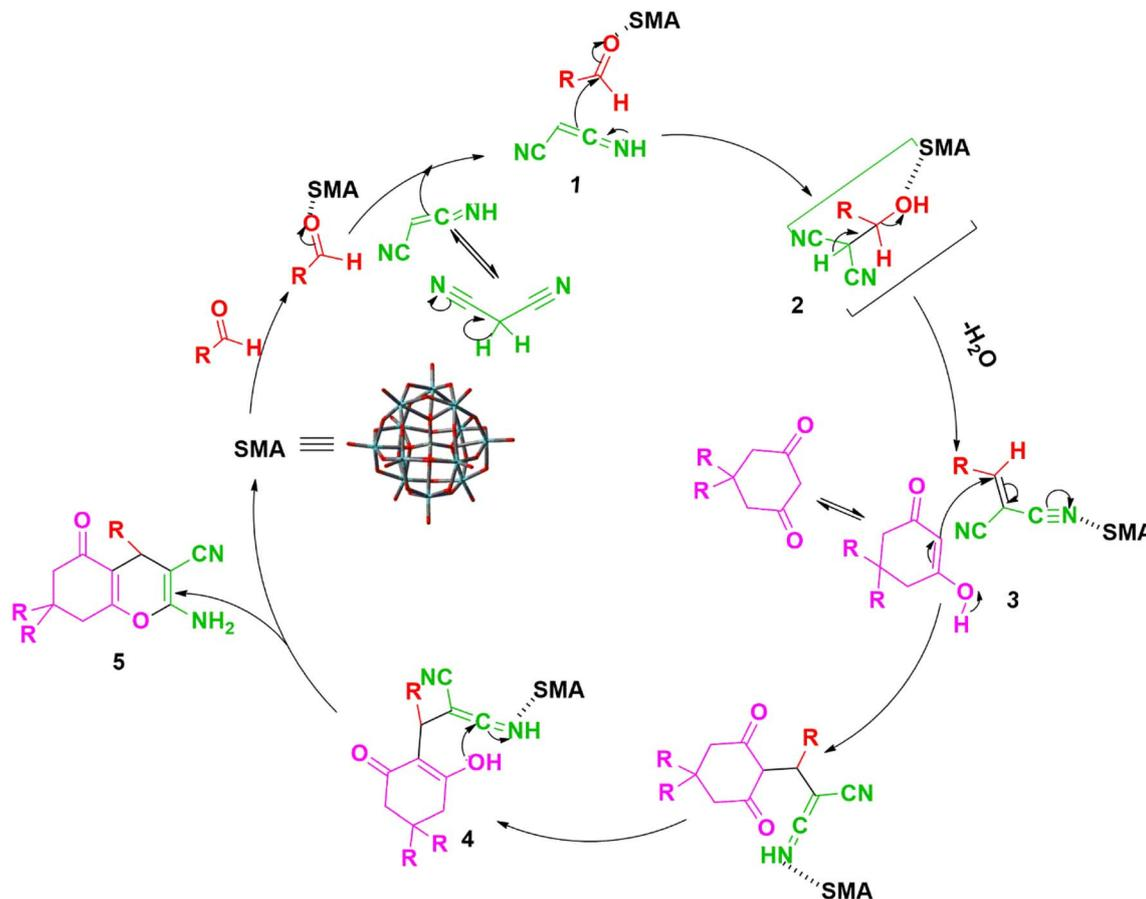
Scheme 2 Schematic mechanism<sup>29</sup> for the catalytic activity of SMA in the synthesis of title compounds (2a–j).
