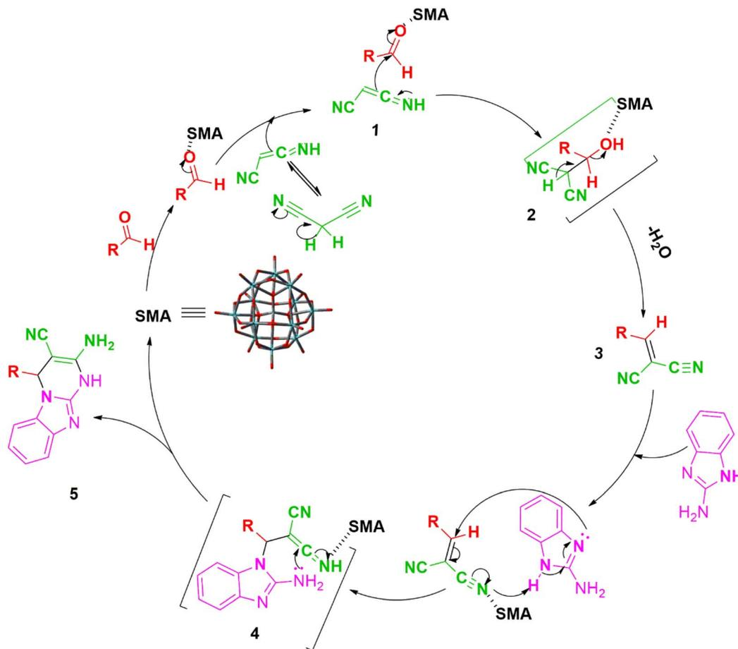
Scheme 3 Schematic mechanism<sup>34</sup> for the catalytic activity of SMA in the synthesis of title compounds (3a–j).Table 9 Comparison of SMA's catalytic efficiency for the synthesis of **3b** with that of other catalytic systems
