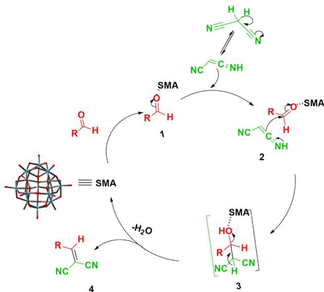
Scheme 1 Schematic mechanism<sup>45</sup> for the catalytic activity of SMA in the synthesis of title compounds (1a–m).
