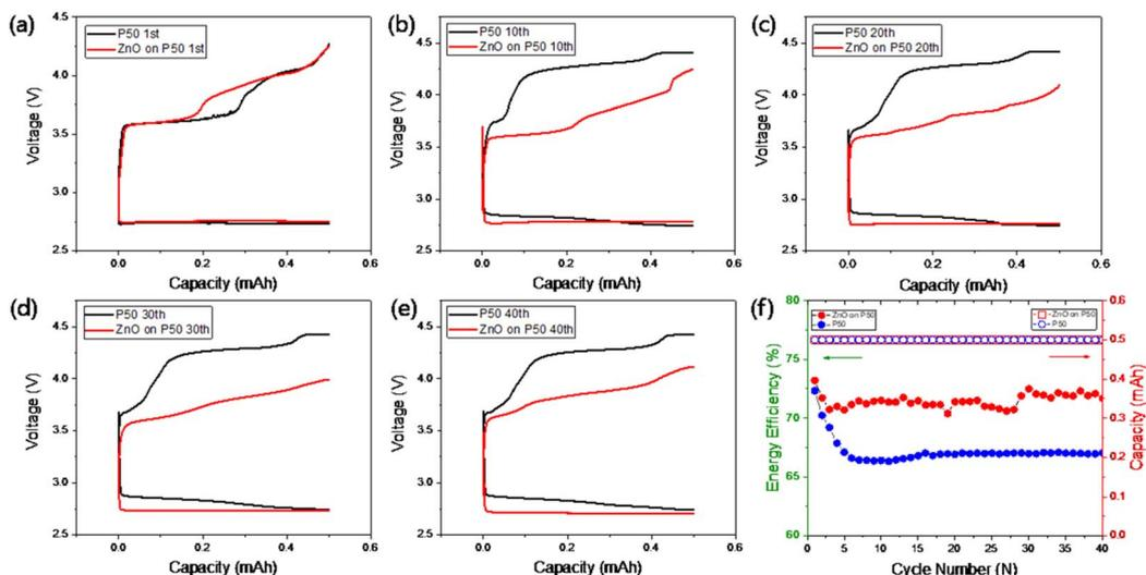
Fig. 7 1st (a), 10th (b), 20th (c), 30th (d) and 40th (e) discharge–charge profiles of the Li–O<sub>2</sub> cell using pristine P50 (black) and ZnO on P50 (red) at a current density of 0.5 mA/h and their cycle performance and energy efficiency (f).
