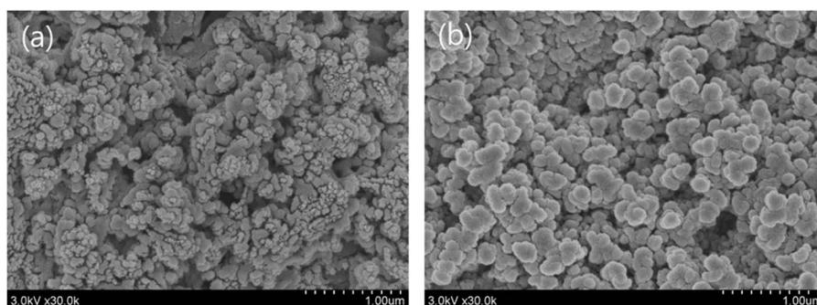
Fig. 9 SEM images of discharge product (Li<sub>2</sub>O<sub>2</sub>): pristine P50 (a), ZnO on P50 (b).
