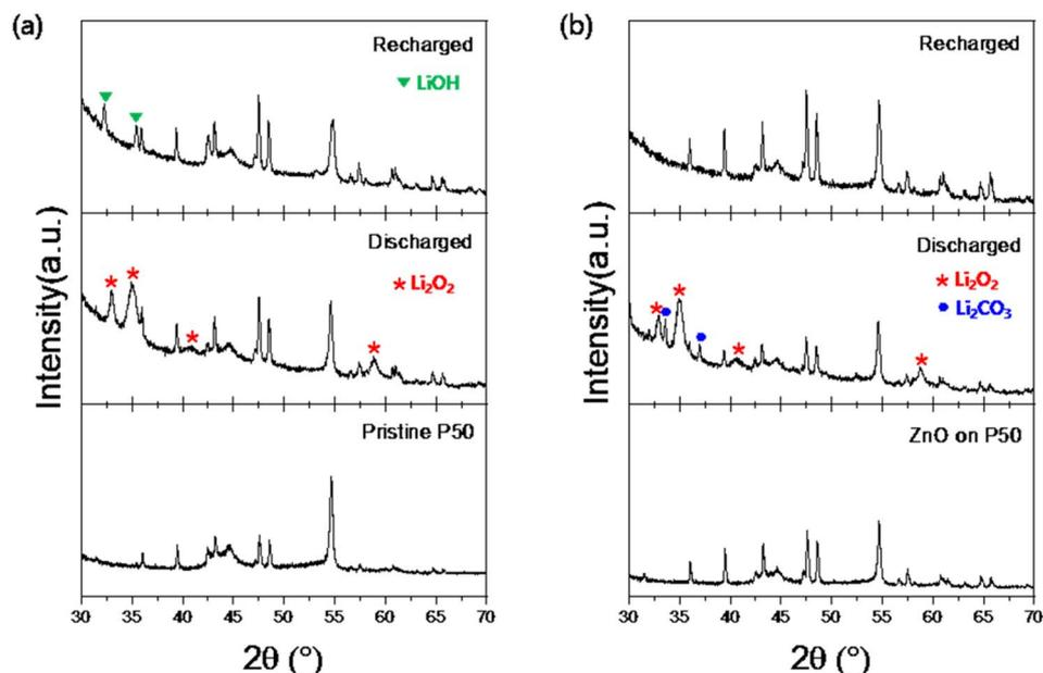
Fig. 8 *Ex situ* XRD patterns at different state of the Li–O<sub>2</sub> cell using pristine P50 (a) and ZnO on P50 (b).
