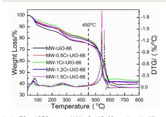
Fig. 5 TG and DTG curves of MW-xCr-UiO-66 samples with different additions of Cr<sup>3+</sup> (molar ratio Cr: Zr = 0, 0.5, 1.0, 1.2, 1.5).
