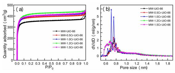
Fig. 6 Nitrogen sorption isotherms (a) and pore size distributions (b) of MW-xCr-UiO-66 samples with different additions of Cr<sup>3+</sup> (molar ratio Cr: Zr = 0, 0.5, 1.0, 1.2, 1.5).
