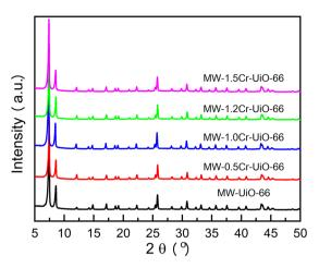
Fig. 2 XRD patterns of MW-xCr-UiO-66 samples with different additions of  $Cr^{3+}$  (molar ratio Cr: Zr = 0, 0.5, 1.0, 1.2, 1.5).
