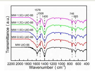
Fig. 3 FTIR curves of MW-xCr-UiO-66 samples with different additions of  $Cr^{3+}$  (molar ratio Cr:  $Zr=0,\,0.5,\,1.0,\,1.2,\,1.5$ ).
