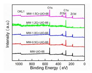
Fig. 4 XPS spectra of MW-xCr-UiO-66 samples with different additions of  $Cr^{3+}$  (molar ratio Cr: Zr = 0, 0.5, 1.0, 1.2, 1.5).
