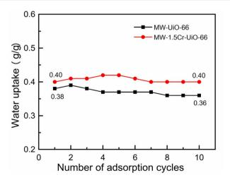
Fig. 8 Water adsorption cycles of MW-UiO-66 and MW-1.5Cr-UiO-66.
