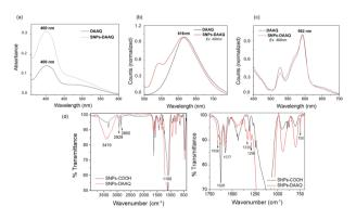
Fig. 2 (a) Comparative UV-vis spectrum for SNPs-DAAQ suspension in ethanol (2 mg mL<sup>-1</sup>), and DAAQ in ethanol solution (1  $\times$  10<sup>-4</sup> M); (b) comparative fluorescence spectroscopy for SNPs-DAAQ suspension in ethanol (2 mg mL<sup>-1</sup>), and DAAQ in ethanol ([DAAQ] =  $1 \times 10^{-4}$  M,  $\lambda_{exc} = 400$  nm); (c) comparative solid-state fluorescence of SNPs-DAAQ and DAAQ; (d) comparative FT-IR analysis for SNPs-COOH (black) and SNPs-DAAQ (red).
