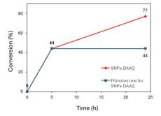
Fig. 5 Filtration test in the dehalogenation of 4-bromobenzonitrile (1a) to benzonitrile (2a) in the presence of SNPs-DAAQ.
