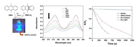
Fig. 7 Photocatalytic oxidation of DMA (6  $\times$  10<sup>-5</sup> M) to 9,10-endoperoxide. Decrease in absorbance of DMA vs. irradiation time using SNPs-DAAQ (10 mol%). Irradiation conditions: Blue LED 3W lamp and EtOH as the solvent.
