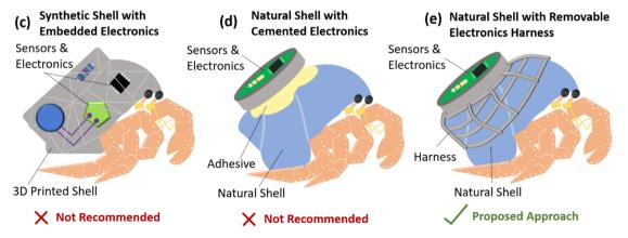
Fig. 1 (a) Anatomy of terrestrial hermit crab. It shows the hardened exoskeleton and soft abdomen. (b) Utilization of an empty gastropod shell where the soft abdomen is protected. Strategies for terrestrial hermit crab to courier sensors and electronics: (c) 3D-printed synthetic shell (not recommended), (d) attaching sensors and electronics via adhesives to natural shell (not recommended), and (e) attaching sensors and electronics via a detachable harness (recommended)
