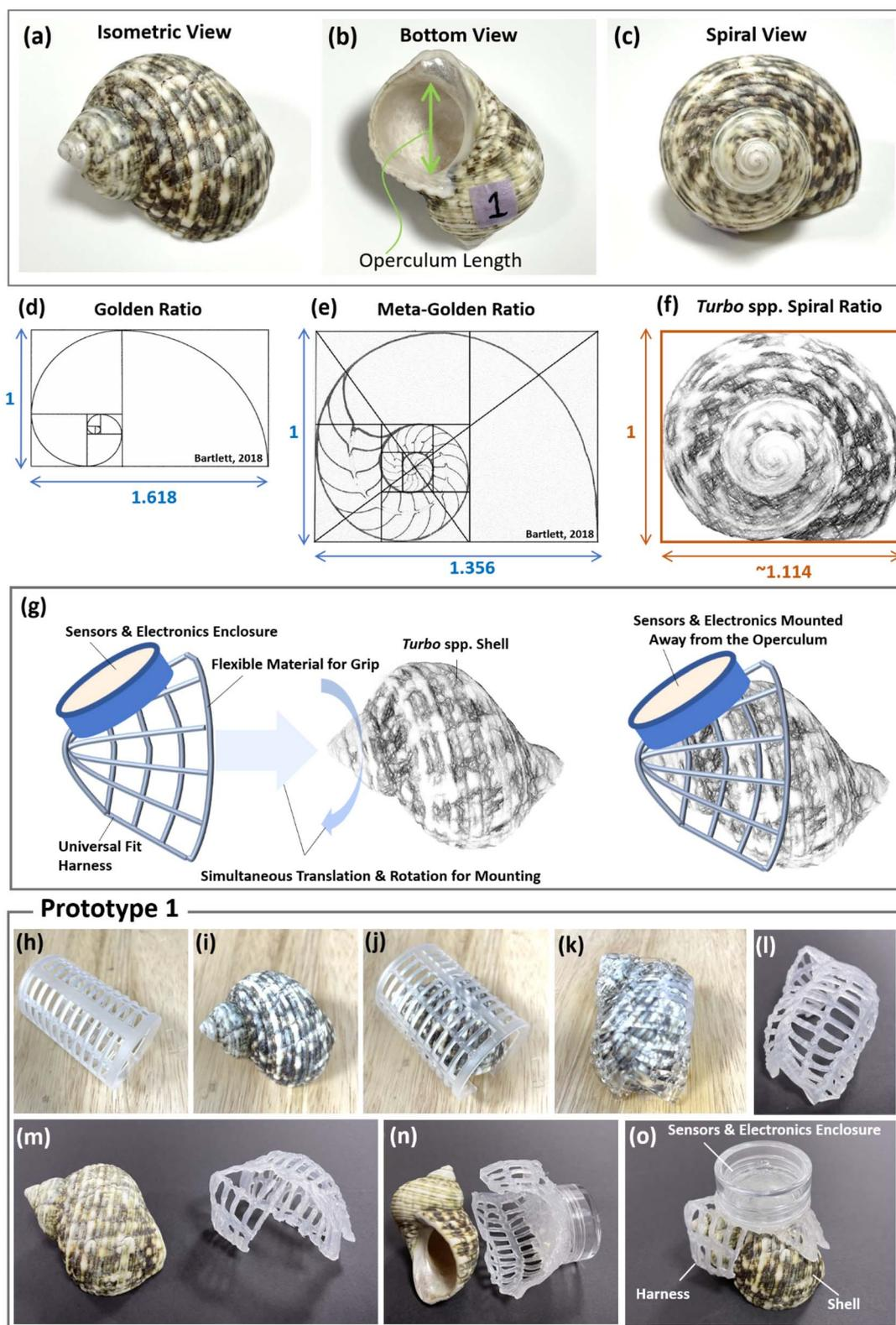
Fig. 2 (a–c) Photographs of natural turbo shells. (d) Golden ratio. (e) Meta-golden ratio. (f) *Turbo* spp. Spiral ratio. (g) Detachable harness conceptual design. (h–o) Step-by-step thermofforming of harness prototype 1 with the sensor and electronic enclosure.
