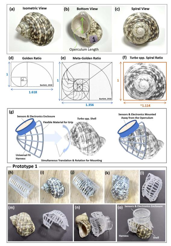
Fig. 2 (a-c) Photographs of natural turbo shells. (d) Golden ratio. (e) Meta-golden ratio. (f) *Turbo* spp. Spiral ratio. (g) Detachable harness conceptual design. (h-o) Step-by-step thermoforming of harness prototype 1 with the sensor and electronic enclosure.
