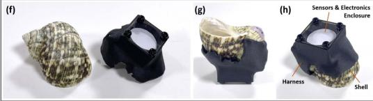
Fig. 3 (a-c) Evolution from harness prototype 1 to 2. (d) Design of harness prototype 2. (e) Key dimensions of harness prototype 2. (f-h) Photographs of harness prototype 2 with the natural shell.
