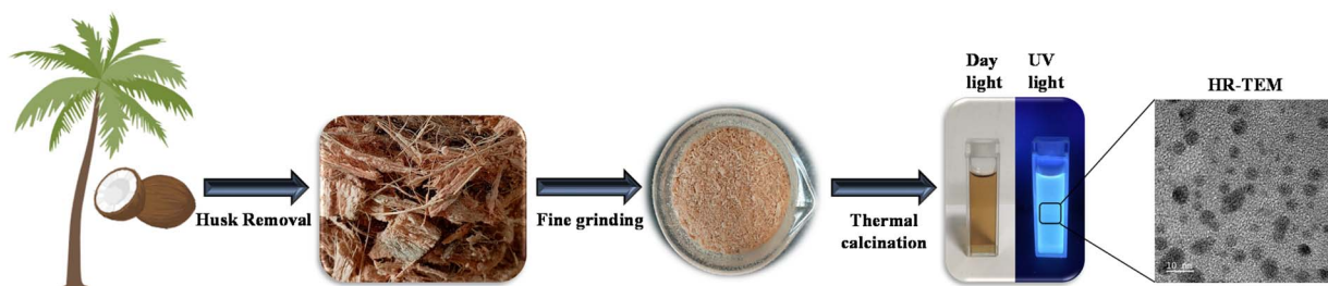
Scheme 1 Schematic of synthesis route for the fluorescent CCDs.
