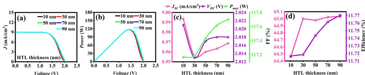
**Fig. 6** (a)  $J$ - $V$  curve, (b)  $P$ - $V$  curve of ZnO/BFO/Spiro-OMeTAD solar cell and effect of HTL's thickness variation on (c)  $J_{sc}$ ,  $V_{oc}$ ,  $P_{max}$  and (d) % FF, % efficiency.
