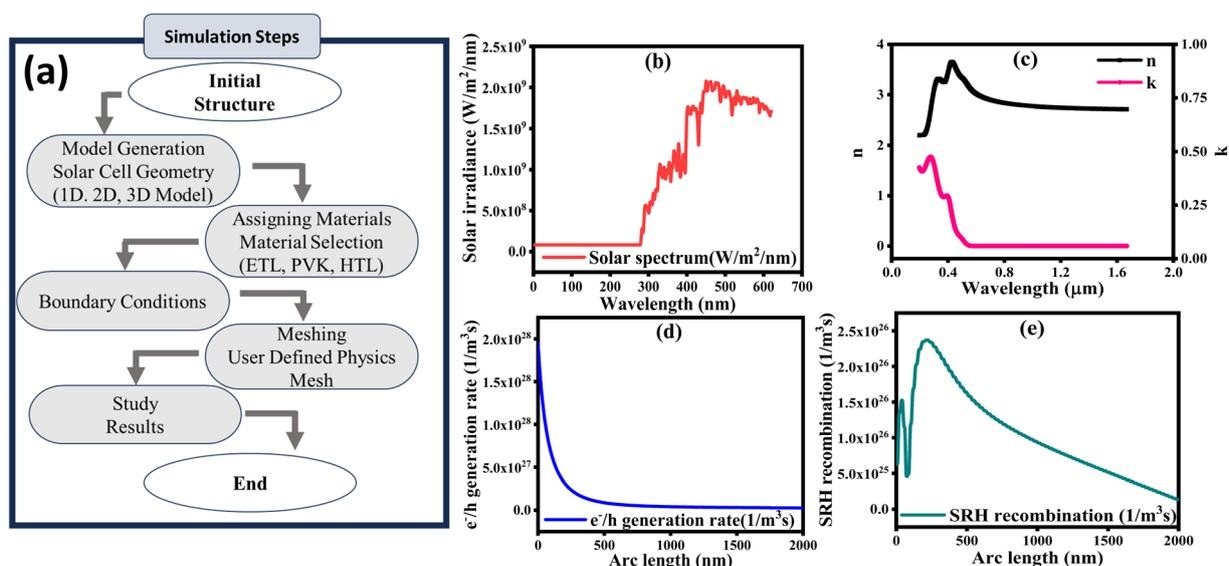
Fig. 1 (a) Flow chart representing the major simulation steps, (b) solar irradiance, (c) solar absorption, (d) electron/hole generation rate and (e) SRH recombination.
