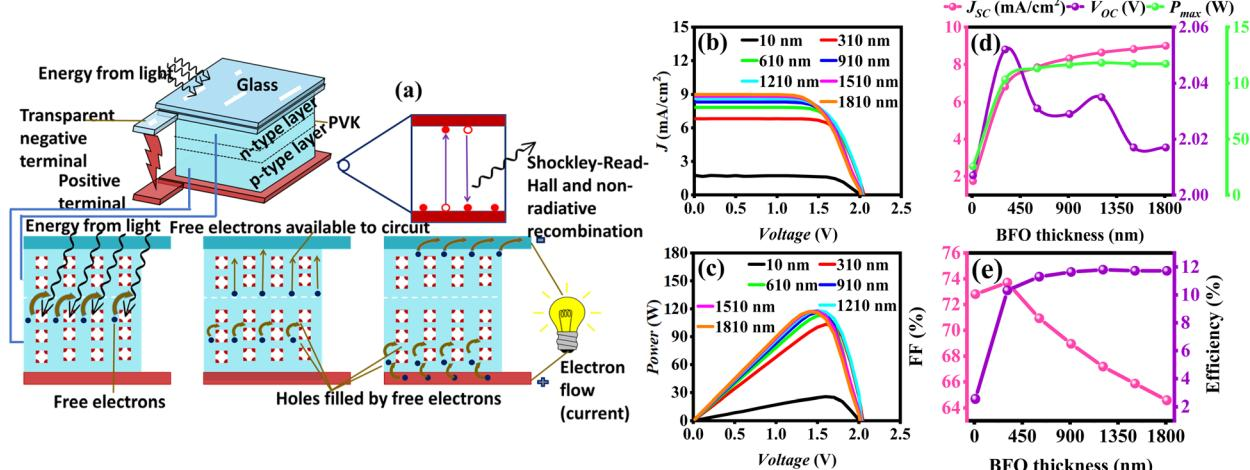
Fig. 4 (a) Schematic illustration of inside working mechanism of photo-induced charge carriers and recombination process, (b)  $J$ – $V$  curve, (c)  $P$ – $V$  curve of ZnO/BFO/Spiro-OMeTAD solar cell and effect of BFO's thickness variation on (d)  $J_{sc}$ ,  $V_{oc}$ ,  $P_{max}$  and (e) % FF and % efficiency.
