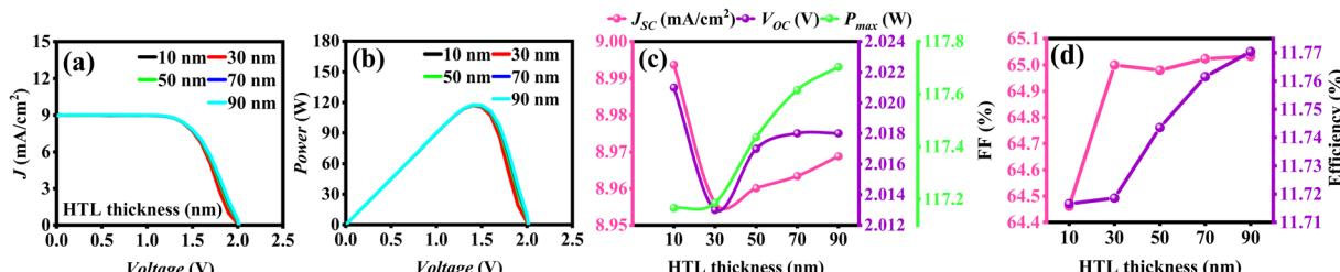
**Fig. 6** (a)  $J$ - $V$  curve, (b)  $P$ - $V$  curve of ZnO/BFO/Spiro-OMeTAD solar cell and effect of HTL's thickness variation on (c)  $J_{sc}$ ,  $V_{oc}$ ,  $P_{max}$  and (d) % FF, % efficiency.
