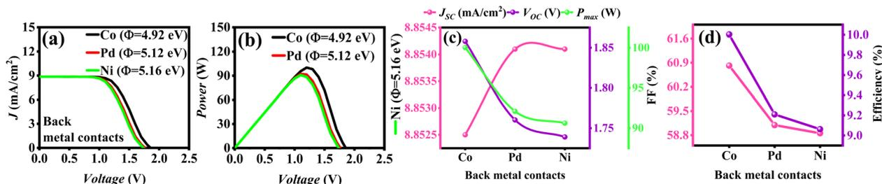
Fig. 7 (a)  $J$ - $V$  curve, (b)  $P$ - $V$  curve of ZnO/BFO/Spiro-OMeTAD solar cell and effect of metal work function variation on (c)  $J_{sc}$ ,  $V_{oc}$ ,  $P_{max}$  and (d) % FF and % efficiency.
