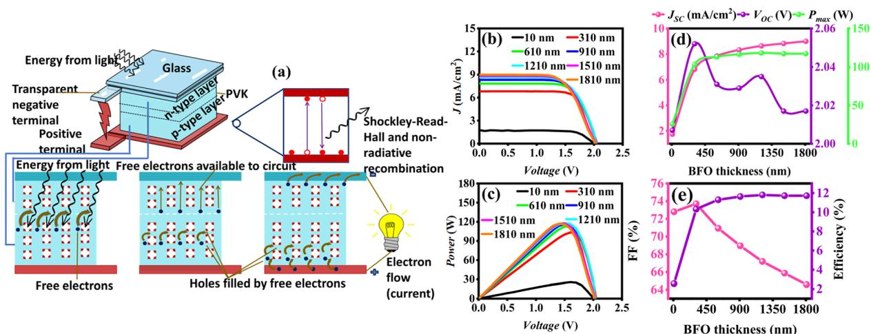
Fig. 4 (a) Schematic illustration of inside working mechanism of photo-induced charge carriers and recombination process, (b)  $J$ - $V$  curve, (c)  $P$ - $V$  curve of ZnO/BFO/Spiro-OMeTAD solar cell and effect of BFO's thickness variation on (d)  $J_{sc}$ ,  $V_{oc}$ ,  $P_{max}$  and (e) % FF and % efficiency.
