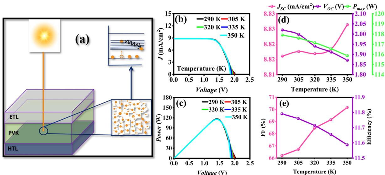
Fig. 8 (a) Schematic illustration of the effect of increased temperature on charge carrier mobility and resistance in the solar cell, (b)  $J$ - $V$  curve, (c)  $P$ - $V$  curve of ZnO/BFO/Spiro-OMeTAD solar cell and effect of temperature variation on (d)  $J_{sc}$ ,  $V_{oc}$ ,  $P_{max}$  and (e) % FF and % efficiency.
