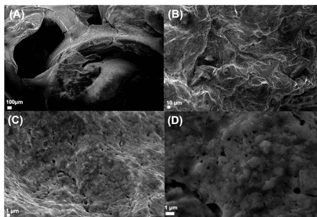
Fig. 5 SEM images of the synthesized hydrogel beads; with scale bars and magnifications at (A) 100  $\mu\text{m}$ , 75 000 $\times$  (B) 10  $\mu\text{m}$ , 500 000 $\times$  (C) 1  $\mu\text{m}$ , 5000 $\times$  and (D) 1  $\mu\text{m}$ , 15 000 $\times$
