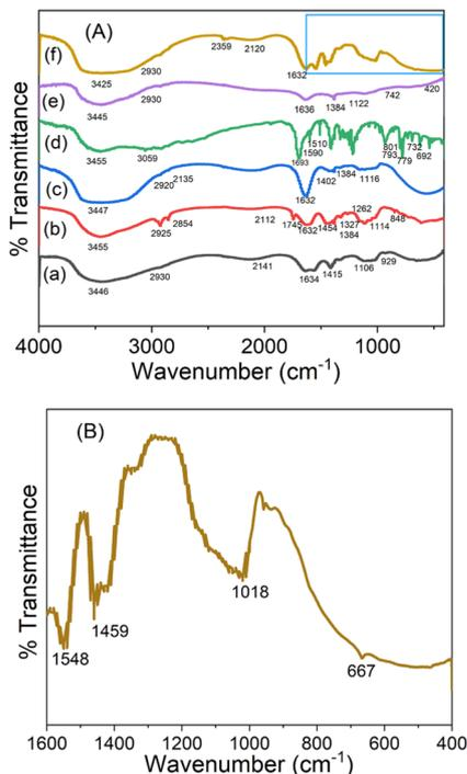
Fig. 6 (A) FTIR spectra of (a) SA, (b) CMC; (c) Ca<sup>2+</sup> crosslinked SA-CMC, (d) NAA; (e) SA-CMC loaded with ZnO NPs; and NAA (f) SA-CMC loaded with ZnO NPs, NAA, and KCl. (B) FTIR spectrum of hydrogel beads in the range 1600–400 cm<sup>-1</sup>.
