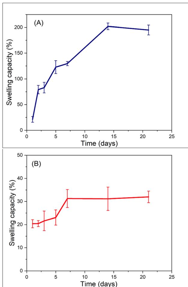
Fig. 7 Swelling capacity of the (A) hydrogel and (B) SA-CMC beads.
