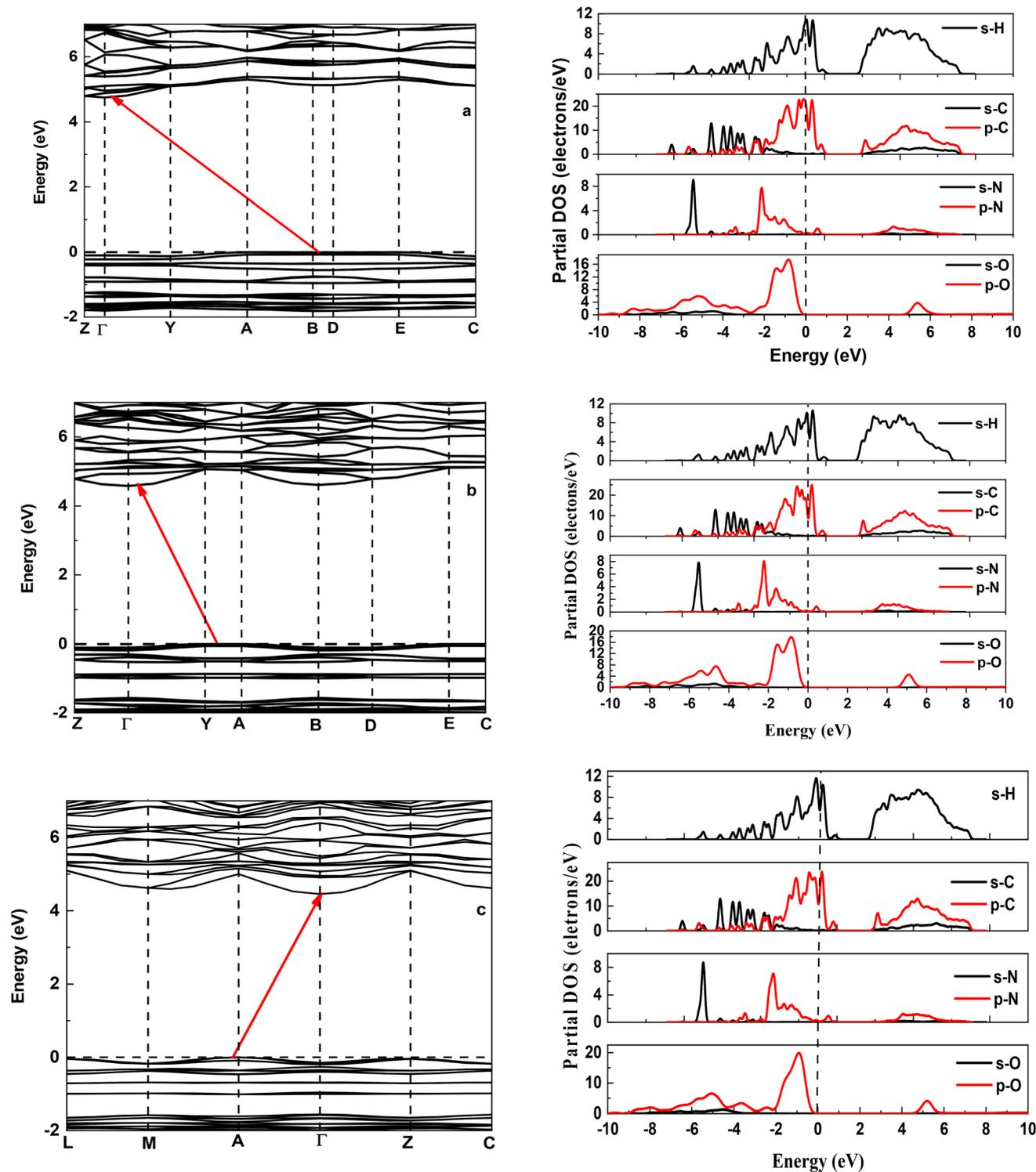
Fig. 2 Band structure and PDOS of the three polymorphs: ( $\alpha$ ) gabapentin (a), ( $\beta$ ) gabapentin (b) and ( $\gamma$ ) gabapentin (c).
