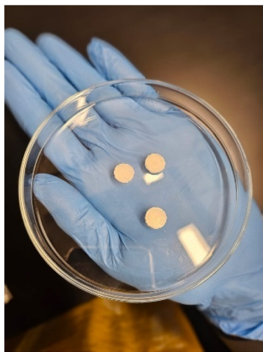
Fig. 2 A picture shows the dimensions of the obtained/fabricated electrode samples for sensing electrophysiological signal.
