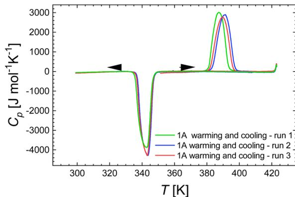
Fig. 9 DSC measurements for  $[\text{Fe}(\text{Htrz})_2\text{trz}]\text{BF}_4$  (**1**) over the 300–423 K temperature range, at a scan rate of  $10 \text{ K min}^{-1}$ , in cooling and warming modes, for three consecutive runs.
