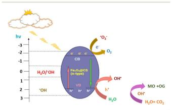
Fig. 6 Illustration of MO and OG dye molecule oxidation after e<sup>-</sup>-h<sup>+</sup> production on a Fe<sub>2</sub>O<sub>3</sub>@CS photocatalyst.
