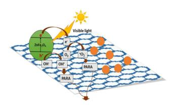
Fig. 8 A graphical representation of PARA's photocatalytic degradation over the  $ZnFe_2O_4-x$  wt% GR nano-hybrid.
