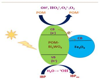
Fig. 10  $\,$  A schematic illustration of the IBP photocatalytic reaction on the Fe  $_3{\rm O}_4/{\rm Bi}_2{\rm WO}_6$  nanohybrid.
