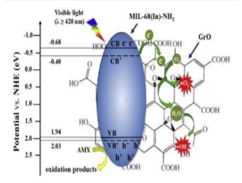
Fig. 9 Photocatalytic mechanism of MIL-68(In)-NH $_2$ /GO composite. This figure has been adapted from ref. 160 with permission from Elsevier, copyright 2017.
