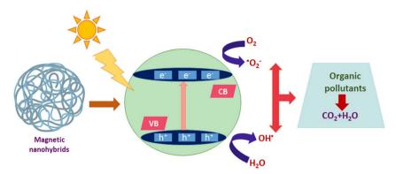
Fig. 5 General mechanism for organic dye degradation by photocatalysis.
