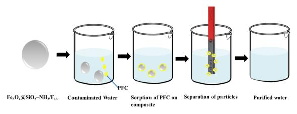
Fig. 2 Removal of PFC particles from surface water using Fe<sub>3</sub>O<sub>4</sub>@SiO<sub>2</sub>-NH<sub>2</sub>/F<sub>13</sub> magnetic hybrid composite. This figure has been reproduced from ref. 113 with permission from Elsevier, copyright 2016.
