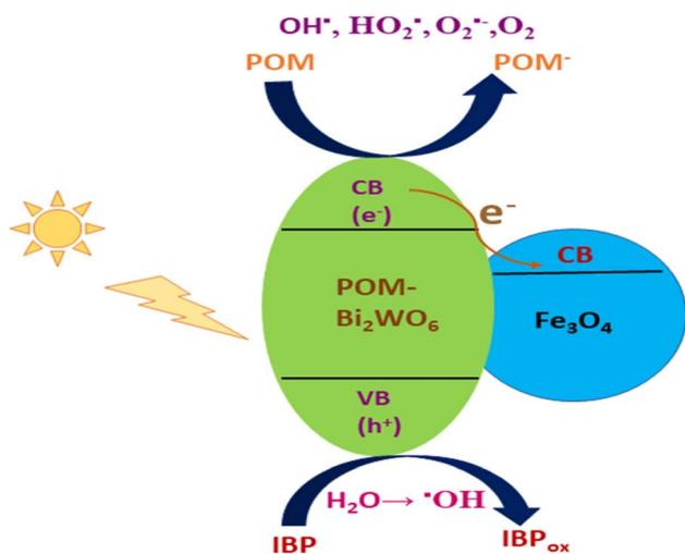
Fig. 10 A schematic illustration of the IBP photocatalytic reaction on the Fe<sub>3</sub>O<sub>4</sub>/Bi<sub>2</sub>WO<sub>6</sub> nanohybrid.
