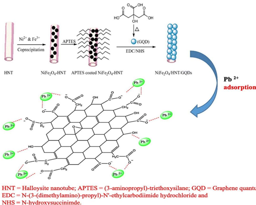
Fig. 4 Synthesis of NiFe<sub>2</sub>O<sub>4</sub>/HNTs/GQDs and plausible adsorption mechanism of Pb(II) ions onto NiFe<sub>2</sub>O<sub>4</sub>/HNTs/GQDs. This figure has been adapted from ref. 130 with permission from Elsevier, copyright 2020.
