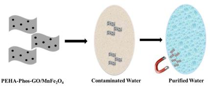
Fig. 3 Removal of lead ions using PEHA-Phos-GO/MnFe<sub>2</sub>O<sub>4</sub> nanohybrid.
