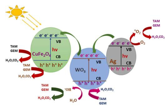
Fig. 11 Photodegradation mechanism of the Ag-CuFe<sub>2</sub>O<sub>4</sub>@WO<sub>3</sub> nanoparticles in the drug models.
