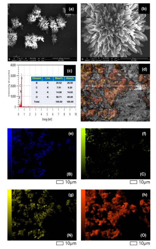
Fig. 5 (a and b) FESEM images taken at different magnifications, (c) EDAX spectrum, and (d-h) elemental mapping images of the BCNO phosphor.
