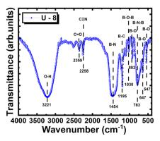
Fig. 3 FTIR spectra of the BCNO phosphor.
