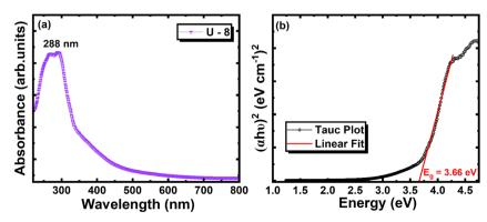
Fig. 6 (a) UV-Vis DRS spectra and (b) Tauc plot of the BCNO phosphor.
