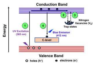
Fig. 9 Afterglow mechanism of BCNO phosphor.
