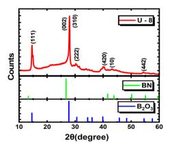
Fig. 2 XRD pattern of the BCNO afterglow phosphor with corresponding JCPDS cards of BN and B2O3.
