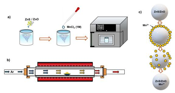
Fig. 1 (a and b) Schematic of the ZnS/ZnO:Mn<sup>2+</sup> fabrication process; (c) illustration of the Mn<sup>2+</sup> diffusion mechanism.
