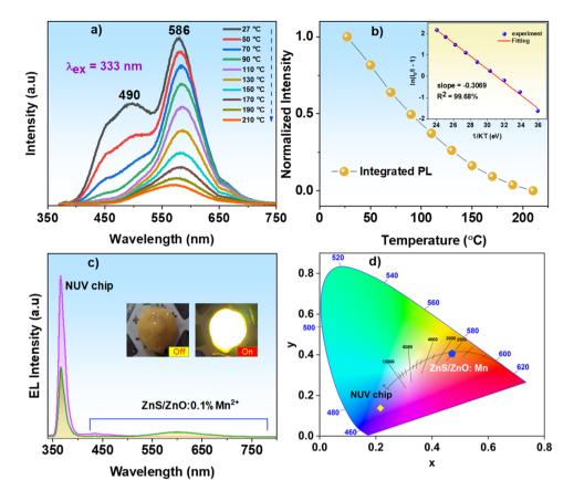
Fig. 10 (a) The temperature-dependent PL spectra excited at 333 nm of ZnS/ZnO:0.1% Mn<sup>2+</sup> phosphors, (b) the corresponding integral normalized PL intensity as a function of temperature. (c) EL spectra of the NUV chip (366 nm) without and with coating a layer of the ZnS/ZnO:0.1% Mn<sup>2+</sup> phosphor and (d) color coordinates of the fabricated LED.
