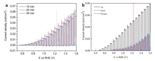
Fig. 6 Chopped LSV curves of GZO samples (a) deposited at various deposition times and (b) annealed at 500 °C in air, nitrogen and argon environments after deposition.
