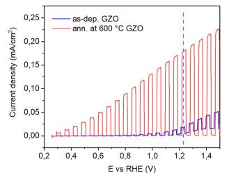
Fig. 8 Chopped LSV curves of as-deposited and annealed at 600  $^{\circ}\text{C}$  GZO samples.
