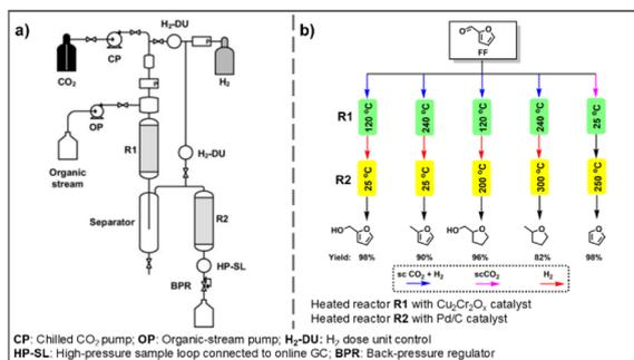
Fig. 3 (a) Automated continuous-flow apparatus diagram. (b) Product distribution with simple modulation of temperature and/or H<sub>2</sub> pressure.
