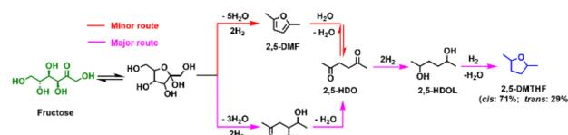
Scheme 6 Suggested mechanism for the reductive valorisation of fructose into 2,5-DMTHF.
