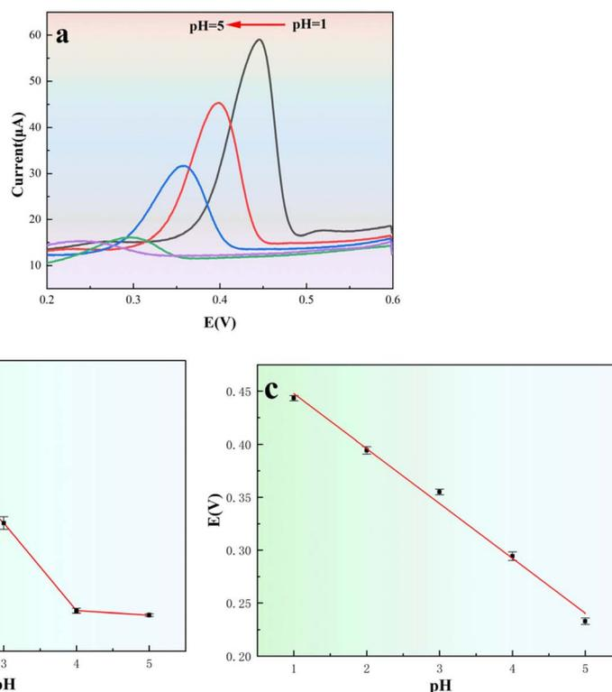
Fig. 8 (a) Effect of PBS with different pH values on the peak current and peak potential of CM. (b) Relationship between different pH values and peak current. (c) Linear relationship between different pH values and peak potential.
