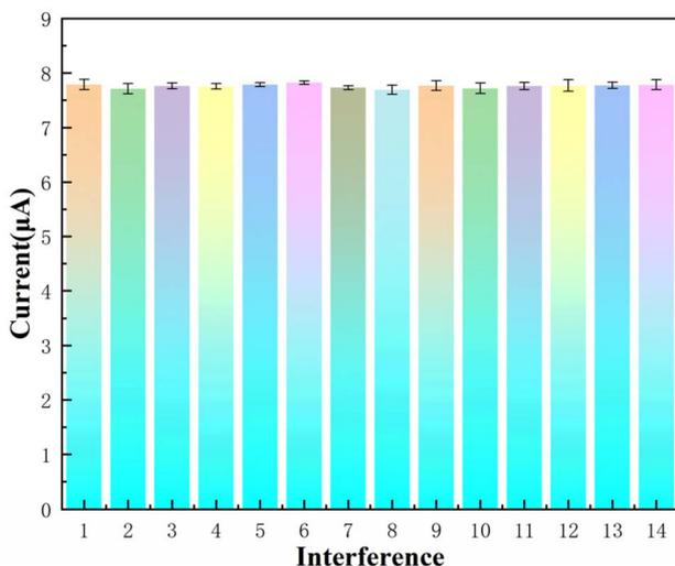
Fig. 11 LSV response of CM in 0.1 M PBS solution at pH = 5.0 at CTPSI-PC/GCE for different interfering compounds.
