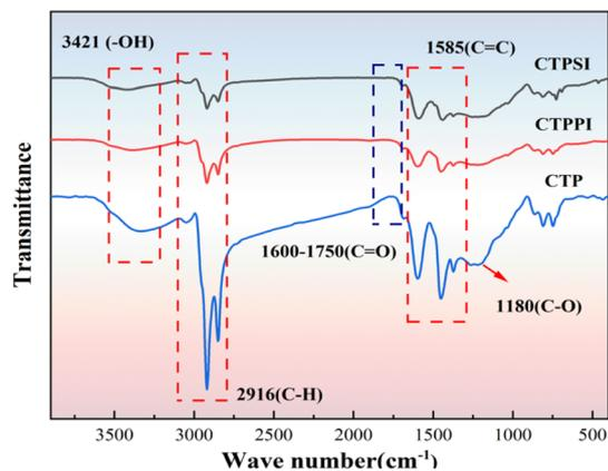
Fig. 2 FT-IR spectra of CTP, CTPPI and CTPSI.
