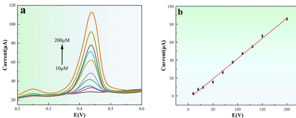
Fig. 10 (a) LSV curves of CM at CTPSI-PC/GCE (0.1 M PBS, pH = 1.0) for different CM concentrations (10, 20, 30, 50, 70, 90, 110, 130, 150 and 200  $\mu\text{M}$ ). (b) Linear relationship between CM concentration and peak current.
