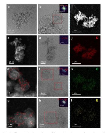
Fig. 6 Characterization of uranyl ion adsorption on the surface of nanodiamonds. (a) Low magnification TEM image showing the morphology of raw nanodiamonds; (b) high magnification TEM image with FFT pattern showing the crystalline structure of nanodiamonds; (c-h) HAADF and BF STEM images showing the monodispersed uranium atomic sites on the surface of nanodiamonds; (i-l) EDS mapping of uranyl ions absorbed nanodiamonds.
