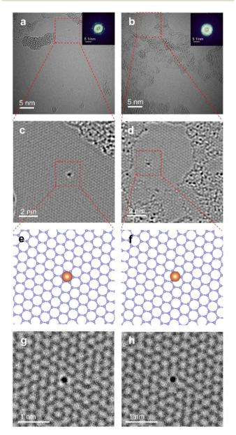
Fig. 4 Two characteristic configurations of monodispersed uranium atomic site on pristine graphene. (a and b) AC-TEM images of uranium atom located at the hollow site and at the top site of carbon atom of graphene; (c and d) enlarged and filtered AC-TEM images of (a) and (b); (e and f) atomic models of uranium atoms of (c) and (d); (g and h) QSTEM simulated TEM image of atomic models of (q) and (h).
