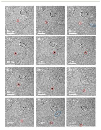
Fig. 5 Migration of uranium atoms at the edge of graphene under electron beam irradiation over time (the red circle shows a single uranium atom, and the blue ellipse shows graphene nanowires).
