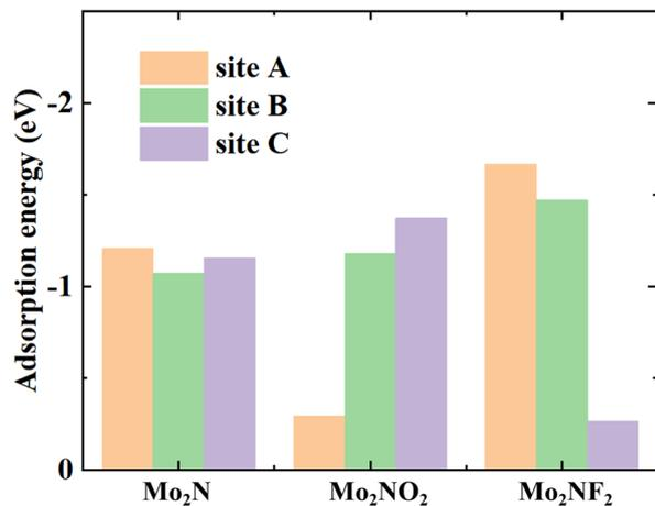
Fig. 2 Calculated adsorption energies of Li at different adsorption sites on monolayers of Mo<sub>2</sub>N and Mo<sub>2</sub>NT<sub>2</sub> (T = F, O).
