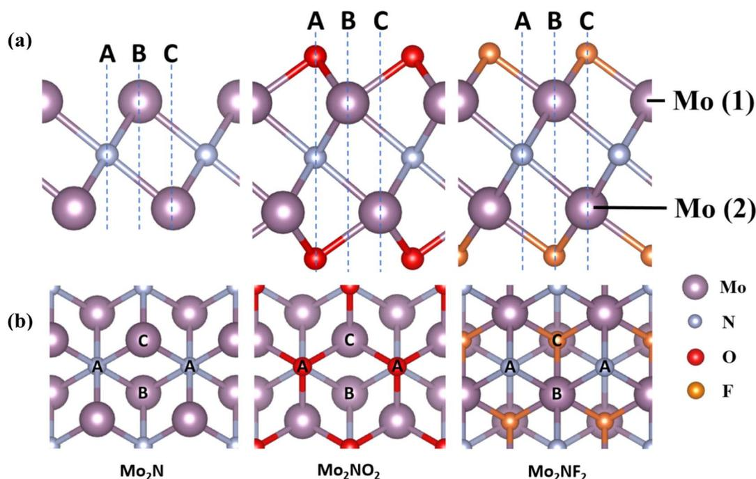
Fig. 1 (a) Side view and (b) top view of the structural model of Mo<sub>2</sub>N and Mo<sub>2</sub>NT<sub>2</sub> (T = O, F). Mo is purple, N is light blue, O is red, and F is orange. A, B, and C are the three different adsorption sites of the Li atom on Mo<sub>2</sub>N and Mo<sub>2</sub>NT<sub>2</sub>.
