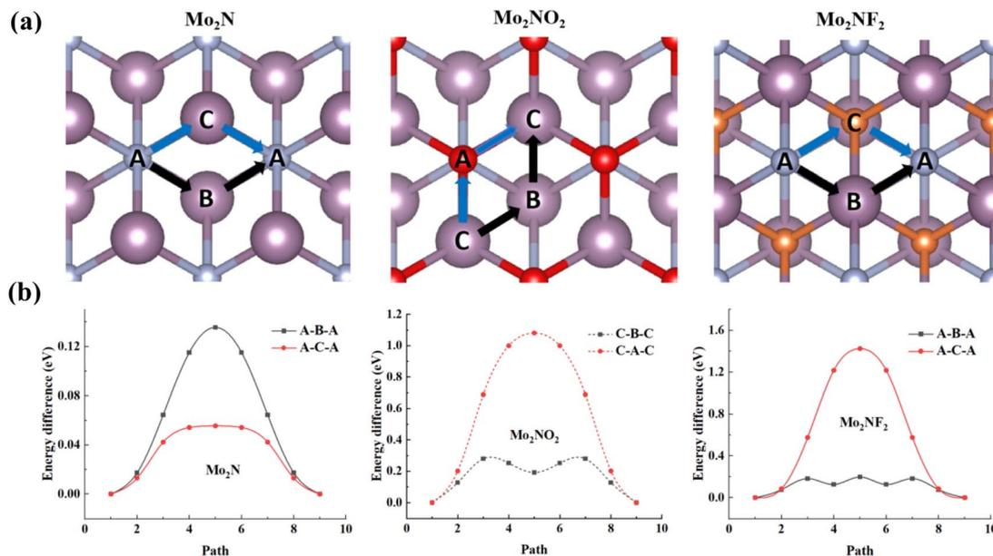
Fig. 5 Lithium diffusion characteristics: (a) schematic representation of minimum energy pathways and (b) corresponding activation energy barriers for Li migration on Mo<sub>2</sub>N, Mo<sub>2</sub>NO<sub>2</sub> and Mo<sub>2</sub>NF<sub>2</sub> surfaces.
