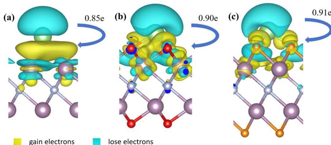
Fig. 3 Charge density difference (CDD) associated with the (a) Mo<sub>2</sub>N (b) Mo<sub>2</sub>NO<sub>2</sub> and (c) Mo<sub>2</sub>NF<sub>2</sub> monolayers after Li atom adsorption, with the yellow iso-surfaces indicating electron gain and blue iso-surfaces indicating electron loss.
