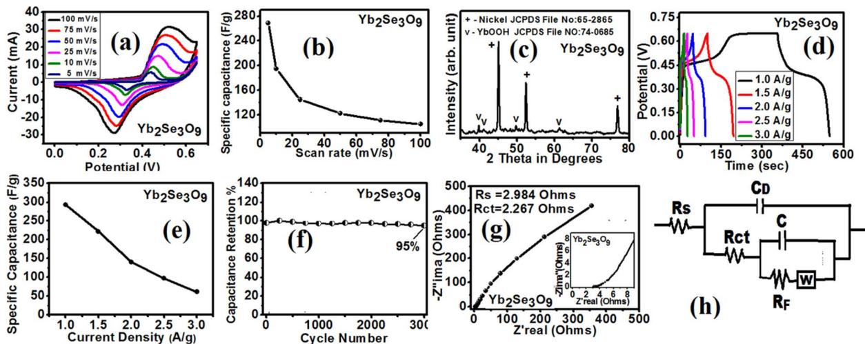
Fig. 5 (a) CV graph, (b) specific capacitance versus scan rate, (c) XRD of  $\text{Yb}_2\text{Se}_3\text{O}_9$  electrode after electrochemical reaction in KOH electrolyte, (d) GCD curves, (e) specific capacitance versus current density, (f) cyclic stability, (g) Nyquist plot and (h) equivalent circuit of  $\text{Yb}_2\text{Se}_3\text{O}_9$ .
