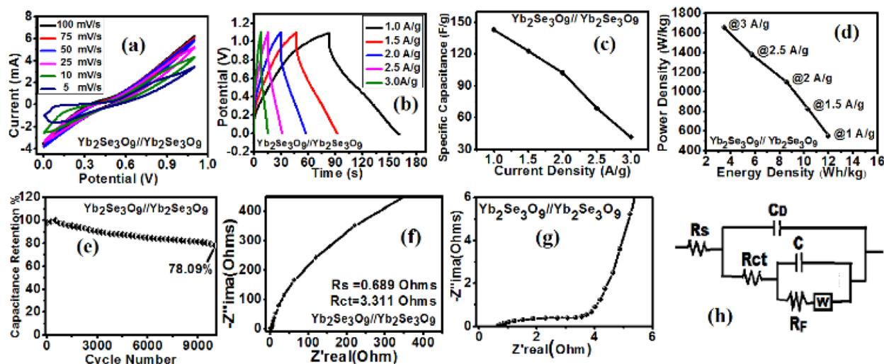
Fig. 6 (a) CV, (b) GCD, (c)  $C_{sp}$  versus current density, (d) Ragone plot, (e) cyclic stability, (f) Nyquist plot, (g) expanded Nyquist plot and (h) equivalent circuit of symmetric  $\text{Yb}_2\text{Se}_3\text{O}_9/\text{Yb}_2\text{Se}_3\text{O}_9$  device.
