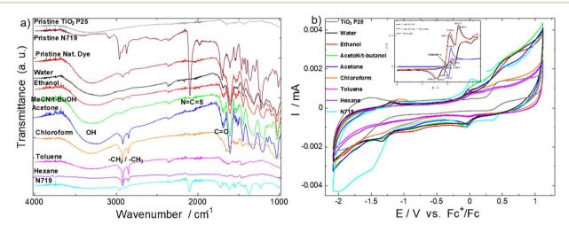
Fig. 7 (a) FT-IR of the natural dyes, N719 dye and pristine  $TiO_2$  P25 nanoparticles from the photoanodes to show essential functional groups for DSSC application and nuanced differences among the natural dye extracts. (b) Cyclic voltammetry plots of the dyes scraped from the photoanodes and deposited on GC electrodes; inset: CV of pristine  $I^-/I_3^-$  electrolyte (black curve), ferrocene + electrolyte, and pristine ferrocene (blue curve) as reference.
