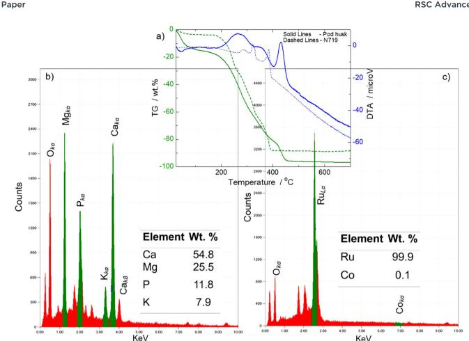
Fig. 4 (a) (overlay on (b) and (c)) TG-DTA (1 °C min<sup>-1</sup>) curves of the pod husk powder showing it's thermal stability, comparable to that of 719 dye powder; (b) and (c) SEM-EDS spectra and tabulated quantitative values (inserts) of residue powders from the TG-DTA characterizations showing their inorganic elemental compositions
