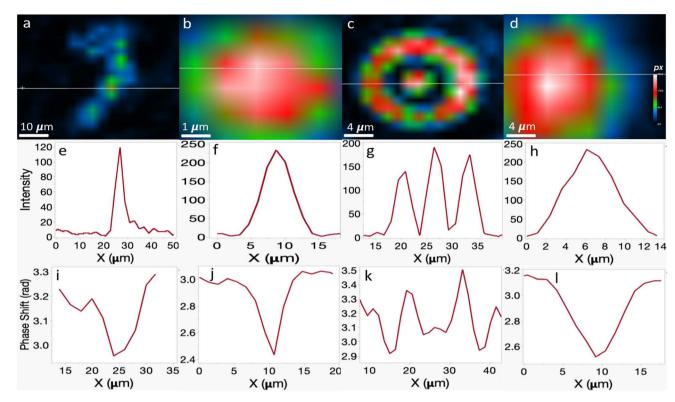
Fig. 5 Reconstruction of airborne CNT particles: (a–d) Intensity reconstructions of different airborne CNT particles, showing circular to elongated morphologies. (e–h) Intensity profiles through the particles' crosscuts, and (i–l) show the phase profiles through the particles' crosscuts. Differences from stationary CNT morphology (Fig. 2) reflect deformation during aerosolization. Al-Nano-DIHM successfully captures airborne CNTs in dynamic environments.
